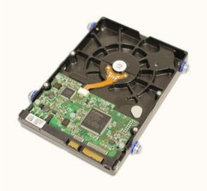
The **hard drive** on your computer is where the software is installed, and it's also where your documents and other files are stored. The hard drive is **long-term storage**, which means the data is still saved even if you turn the computer off or unplug it.
