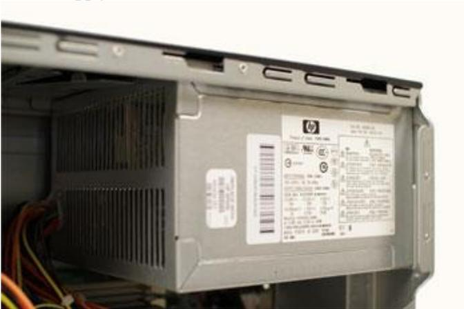
The power supply unit in a computer **converts the power** from the wall outlet to the type of power needed by the computer. It sends power through cables to the motherboard and other components.
