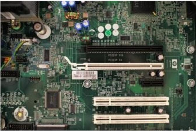
The **motherboard** is the computer's **main circuit board**. It's a thin plate that holds the CPU, memory, connectors for the hard drive and optical drives, expansion cards to control the video and audio, and connections to your computer's ports (such as USB ports). The motherboard connects directly or indirectly to every part of the computer.
