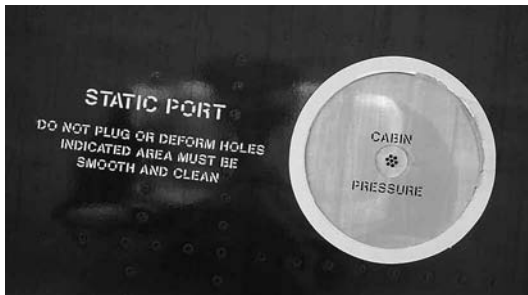
1.12 An aircraft static port
