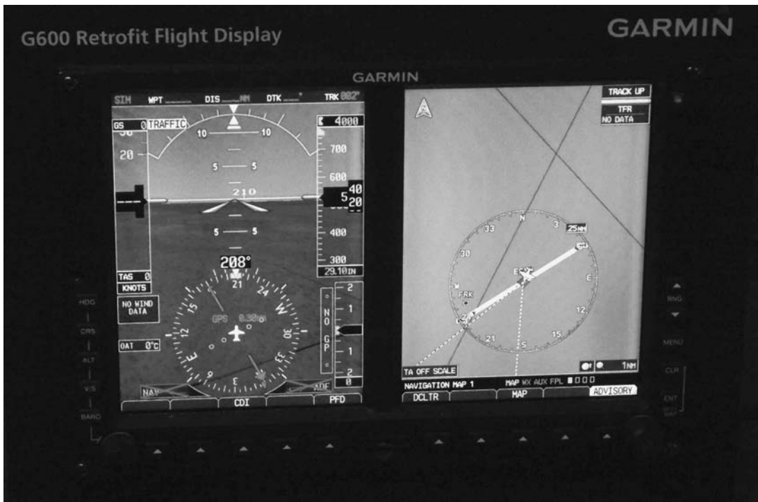
11.18 A colour LCD display in a retrofit instrument system from Garmin
