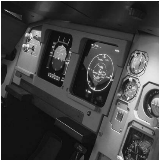
15.3 'Glass cockpit' (EFIS) displays in an A320
