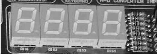
11.13 Typical example of a four-digit seven-segment display
