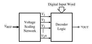
**Figure 9.2-6** General voltage scaling DAC.
