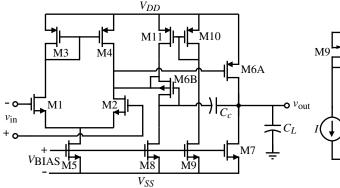
Figure P6.3-13 Nulling resistor implemented by an MOS diode.
