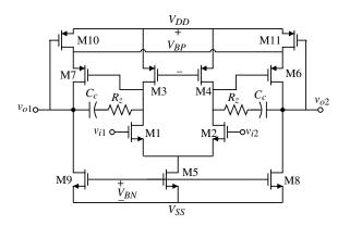
**Figure 7.3-14** Two-stage Miller differential-in, differential-out op amp with common-mode stabilization
