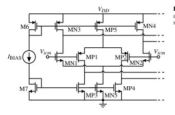
**Figure 7.6-4** Parallel n-channel and p-channel differential input stage.
