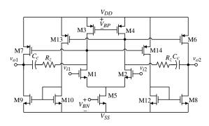
**Figure 7.3-5** Two-stage Miller differential-in, differential-out op amp with a push–pull output stage.
