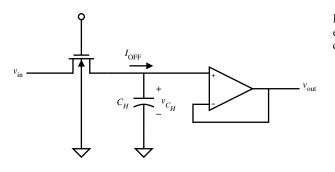
Figure 4.1-8 Example of the influence of  $I_{OFF}$  in a sample-and-hold circuit.
