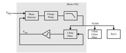
Figure 1.4-3 Master filter phase-locked loop.
