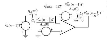
**Figure E.3-10** Equivalent circuit for the noninverting integrator at the beginning of the  $\phi_2$  phase period.
