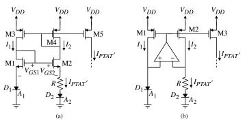
Figure 4.6-3 Creation of pseudo-PTAT currents using (a) MOSFETs only and (b) MOSFETs and an op amp.
