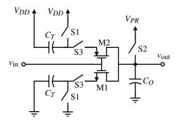
Figure 8.6-7 A CMOS charge-transfer preamplifier.
