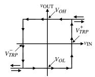
Figure 8.4-5 Comparator transfer curve with hysteresis.
