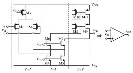
Figure 6.1-9 Folded-cascode op amp broken into stages.
