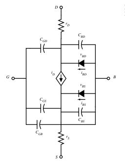
Figure 3.2-1 Complete large-signal model for the MOS transistor.
