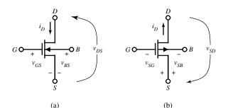
**Figure 3.1-1** Positive sign convention for (a) n-channel and (b) p-channel MOS transistor.
