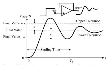
Figure 6.1-7 Transient response of an op amp with negative feedback illustrating settling time  $T_{s}$ .  $\varepsilon$  is the tolerance to the final value used to define the settling time.
