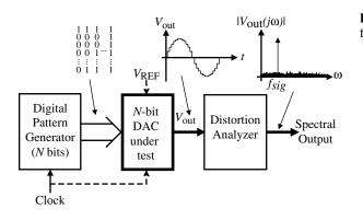
**Figure 9.1-10** Spectral output test for a DAC.
