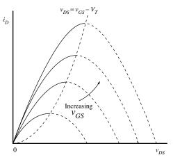
**Figure 3.1-2** Graphical illustration of the modified Sah equation.
