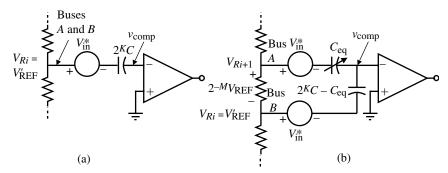
**Figure 9.7-6** (a) Equivalent circuit for the successive-approximation search of the (a) *MSB* subDAC and (b) *LSB* subDAC.
