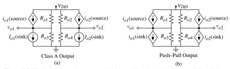
Figure 7.3-12 Common-mode output model for (a) Class A and (b) Class B differentialoutput op amps.
