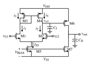
Figure 8.2-3 Two-stage, open-loop comparator used to find initial states.
