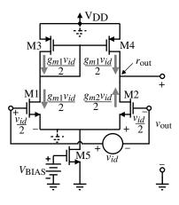
**Figure 5.2-12** Intuitive analysis of the CMOS differential amplifier of Fig. 5.2-6.
