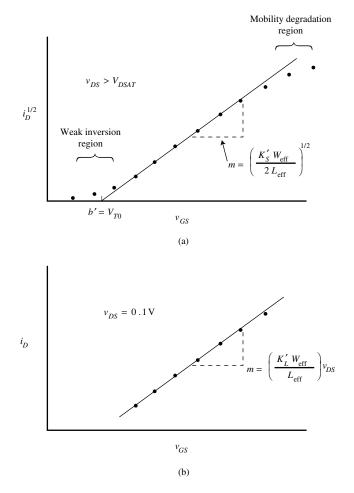
**Figure C.1-1** (a)  $i_{D}^{1/2}$  versus  $v_{GS}$  plot used to determine  $V_{T0}$  and  $K'_{S}$ . (b)  $i_D$  versus  $v_{GS}$  plot to determine  $K'_L$ .
