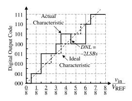
**Figure 9.5-6** Example of nonmonotonic 3-bit ADC.
