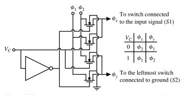
**Figure E.3-8** A circuit that changes the  $\phi_1$  and  $\phi_2$  clocks of the leftmost switches of Fig. E.3-4.
