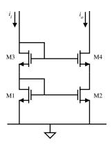
Figure 4.4-6 Standard cascode current sink.
