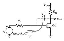
Figure 6.2-9 Illustration of the implementation of the dominant pole through the Miller effect on  $C_c$ . M6 is treated as an NMOS for this illustration.
