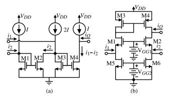
Figure 5.4-7 (a) Current-mirror differential-input current amplifier. (b) Alternate differentialinput current amplifier.
