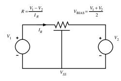
Figure C.4-3 n-Well resistor illustrating backbias dependence.
