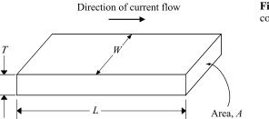
Figure 2.4-4 Current flow in a conductive bar.
