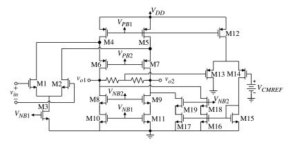
Figure 7.3-16 Improvement of the frequency response of Fig. 7.3-15.
