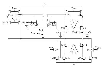
Figure 7.3-9 Enhanced-gain, Class B, folded-cascode, differential-output op amp.
