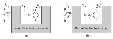
**Figure 4.3-9** (a) Application of Blackman's formula to find the resistance at port X. (b) Circuit used to find the return ratio of Blackman's formula.
