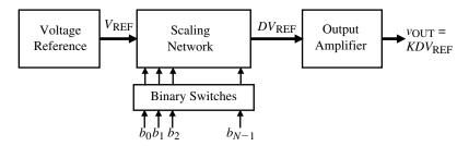
Figure 9.1-3 Block diagram of a digital-analog converter.
