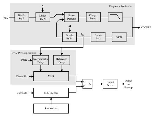
Figure 1.4-4 Frequency synthesizer and write-data path.
