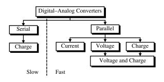
Figure 9.2-1 Classification of digitalanalog converters.
