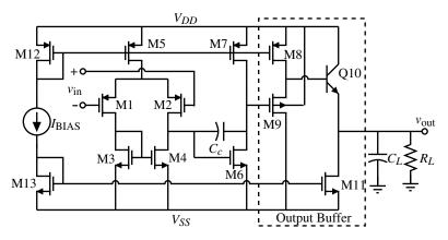
Figure 7.1-11 Two-stage op amp with a Class A, BJT output buffer stage.
