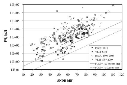
Figure 9.10-1 ADC energy plot of analog-digital converters published from 1997 to 2010 [87].
