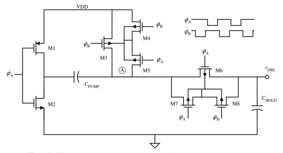
Figure 4.1-14 Voltage doubler used to provide gate overdrive.
