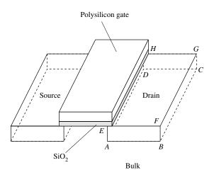
**Figure 3.2-3** Illustration showing the bottom (*ABCD*) and sidewall (*ABFE* + BCGF + DCGH + ADHE) components of the bulk junction capacitors.
