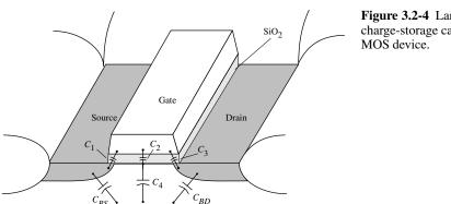
Figure 3.2-4 Large-signal, charge-storage capacitors of the
