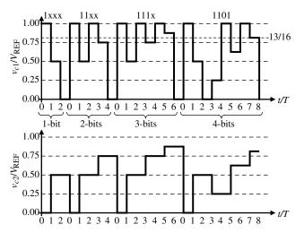
**Figure 9.7-8** Illustration of the operation of the successiveapproximation ADC of Fig. 9.7-7 for the conversion of the sampled analog input voltage of  $\frac{3}{16} V_{\text{REF}}$ . The digital word out is  $b_0 = 1$ ,  $b_1 = 1$ ,  $b_2 = 0$ , and  $b_3 = 1$ .
