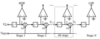
Figure 9.7-9 Pipeline implementation of the algorithmic ADC.
