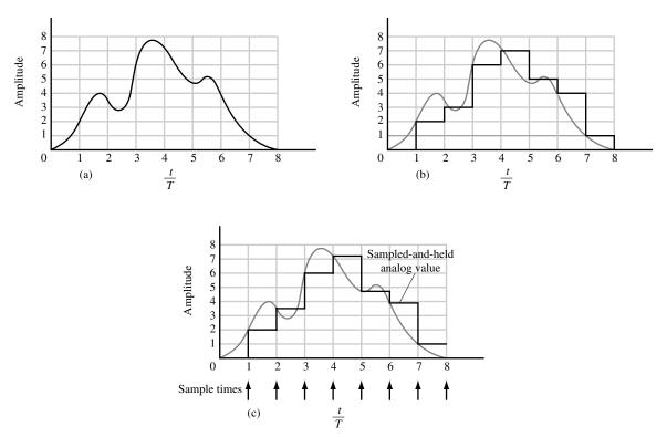
**Figure 1.1-1** Signals. (a) Analog or continuous time. (b) Digital. (c) Analog sampled data or discrete time. *T* is the period of the digital or sampled signals.
