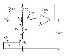
Figure 4.6-7 A realization of the series temperature-independent voltage reference that uses an op amp.
