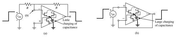
**Figure 5.2-4** (a) Inverting configuration of the op amp with a gain of -1. (b) Noninverting configuration of the op amp with a gain of +1.
