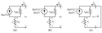
**Figure 4.3-10** (a) Figure 4.3-3(b) with  $v_{g2} = 0$  and  $v_{bs2} = 0$  V. (b) Conversion of Fig. 4.3-10(a) from Fig 4.3-9(a) to Fig. 4.3-9(b), which can also be used for the open-circuit port if  $i_x = 0$ . (c) Short-circuit form of Fig. 4.3-10(b).
