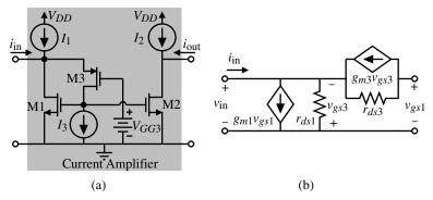
**Figure 5.4-5** (a) Current amplifier using negative shunt feedback to reduce  $R_{in}$ . (b) Small-signal model for calculating  $R_{in}$ .
