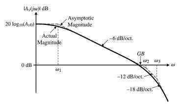
**Figure 6.1-6** Typical frequency response of the magnitude of  $A_{\nu}(j\omega)$  for an op amp.
