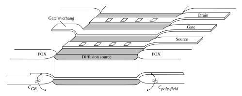
Figure C.5-4 Illustration of gate-to-bulk and poly-field capacitance.
