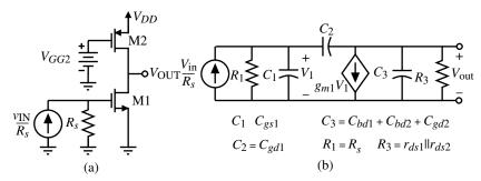
**Figure 5.3-5** (a) Current-source load inverter driven from a high-resistance source. (b) Equivalent small-signal model for (a).
