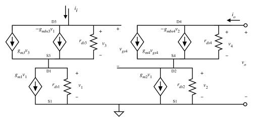
Figure 4.4-7 Small-signal model for the circuit of Fig. 4.4-6.
