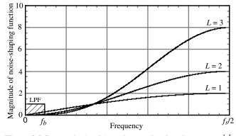
**Figure 9.9-7** Magnitude of the noise-shaping function,  $(1 - z^{-1})^L$ .
