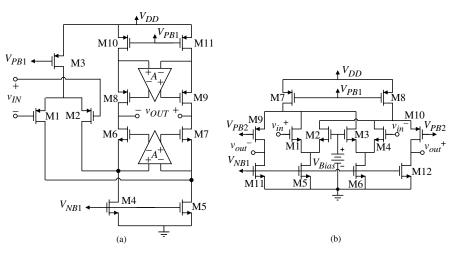
**Figure 7.3-7** (a) Enhanced-gain, folded-cascode, differential-output op amp. (b) Implementation of the upper *A* amplifier.
