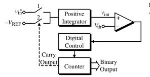
**Figure 9.6-2** Block diagram of a dual-slope ADC.
