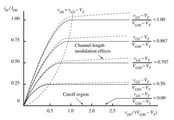
Figure 3.1-3 Output characteristics of the MOS device.
