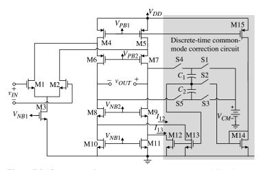
**Figure 7.3-18** Example of a common-mode output voltage stabilization scheme for discrete-time applications.
