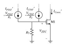
Figure 4.6-13 Implementation of the constant-current generator.
