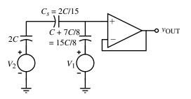
**Figure 9.3-5** Simplified equivalent circuit of Fig. 9.3-4.
