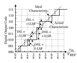
**Figure 9.5-5** Example of *INL* and *DNL* for a 3-bit ADC.
