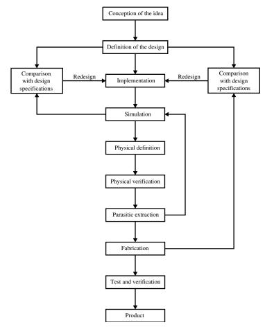
Figure 1.1-3 Design process for analog integrated circuits.
