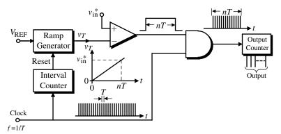
Figure 9.6-1 Block diagram of a single-slope serial ADC.
