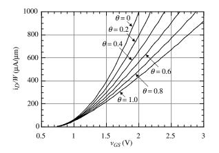
**Figure 3.1-5** Influence of velocity saturation on the transconductance characteristics.
