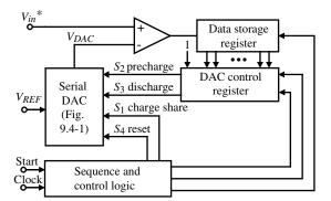
**Figure 9.7-7** A successive-approximation ADC using the serial DAC of Fig. 9.4-1.
