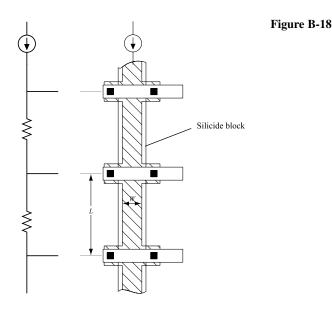
in the R path. This effect can be mitigated by adding vias into the R string or by increasing the value of the resistors so that via resistance is a smaller percentage of the total resistance.
