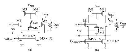
**Figure 5.2-19** Implementation of RS of Fig. 5.2-18(b). (a) Single MOSFET in triode region. (b) Parallel MOSFET implementation of  $R_S$  with both MOSFETs in the triode region.
