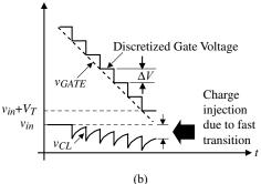
cases, the quantized voltage step,  $\Delta V$ , is the same, but the time between steps is different. The voltage across  $C_L$  is observed to be an exponential whose time constant is due to the channel resistance and channel capacitance and does not change from the fast case to the slow case.
