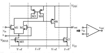
Figure 6.1-8 Classical two-stage CMOS op amp broken into voltage-to-current and current-to-voltage stages.
