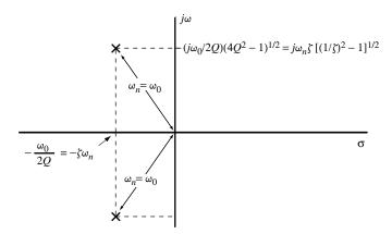
Figure D.1-1 Pole locations of a general second-order system.
