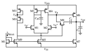
Figure 6.3-4 CMOS two-stage op amp using nulling resistor compensation.
