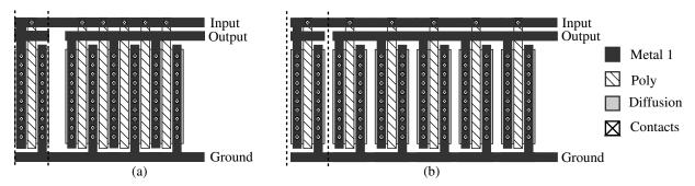
**Figure 6.3-6** The layout of a 5-to-1 current mirror. (a) Layout that minimizes area at the sacrifice of matching. (b) Layout that optimizes matching.
