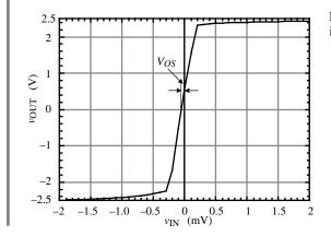
**Figure 6.6-15** Open-loop transfer characteristic of Example 6.6-1 illustrating  $V_{OS}$ .
