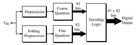
Figure 9.8-7 Architecture of a folding ADC.
