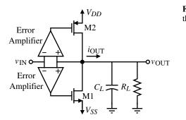
**Figure 5.5-11** Use of negative feedback to reduce the output resistance of Fig. 5.5-8.
