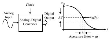
Figure 9.5-14 Illustration of aperture jitter in an ADC.
