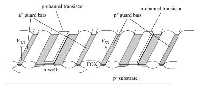
Figure 2.5-4 Preventing latch-up using guard bars in an n-well technology.
