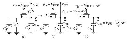
Figure 8.6-6 (a) Charge-transfer amplifier. (b) Precharge phase. (c) Amplification phase.
