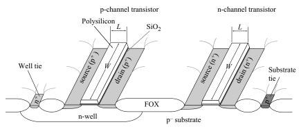
Figure 2.3-1 Physical structure of an n-channel and a p-channel transistor in an n-well technology.
