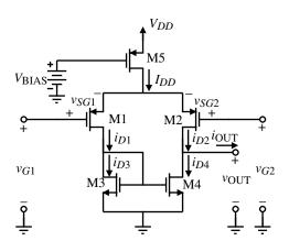
**Figure 5.2-8** CMOS differential amplifier using p-channel input MOSFETs.
