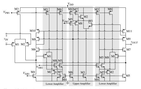
Figure 6.5-16 Complete transistor realization of the enhanced gain folded-cascode op amp.
