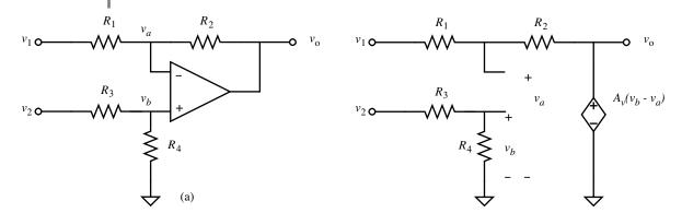
Figure A.1-5 (a) Differential amplifier using an operational amplifier. (b) Small-signal model of (a).
