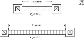
**Figure C.4-2** Two resistors used to determine  $R_S$  and  $R_C$ .
