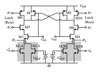
Figure 8.5-6 Comparator using a latch with a built-in threshold.
