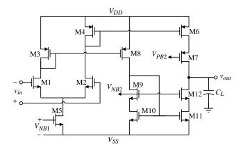
Figure 6.5-6 Op amp using cascode output stage.
