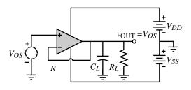
**Figure 6.6-4** Configuration for measuring the input-offset voltage and the simulation of the systematic offset voltage of an op amp.
