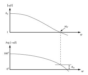
Figure D.3-1 Crossover frequency and phase margin.
