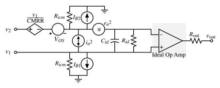
Figure 6.1-5 A model for a nonideal op amp showing some of the nonideal linear characteristics.
