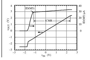
**Figure 6.6-17** Input common-mode simulation of Example 6.6-1.
