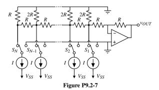
in Fig. P9.2-7. If bit *i* is 1, then switch  $S_i$  is connected to the R-2R ladder; otherwise,  $S_i$  is connected to ground. (a) What is the full scale value of this converter? (b) Design the value of *I* if  $V_{REF} = 5$  V. (c) Assume the worst-case conditions and find the maximum number of bits that this converter can convert at low frequencies if the differential voltage gain of the op amp is given as
