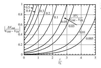
Figure 8.5-5 Normalized timedomain response of a latch.
