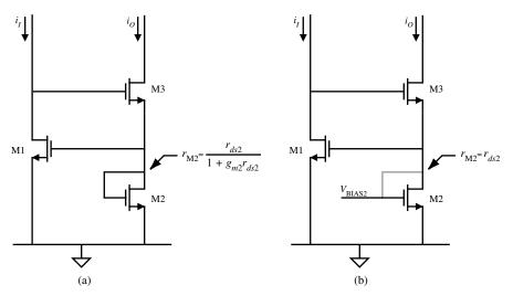
**Figure 4.4-9** (a) Wilson current mirror redrawn. (b) Wilson current mirror modified to increase  $r_{\text{out}}$  at M2.
