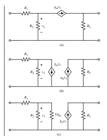
**Figure A.1-8** Current-source rearrangement and substitution. (a) Original circuit. (b) Rearrangement. (c) Substitution.
