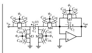
**Figure E.2-9** Noninverting switched capacitor voltage amplifier showing the MOSFET switch overlap capacitors, *C*<sub>0L</sub>.
