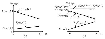
**Figure 4.6-1** (a) Illustration of voltages that increase and decrease with increasing temperature. (b) Multiplication of  $V_{PTAT}(T)$  by *K* to make the slopes of  $V_{PTAT}(T)$  and  $V_{CTAT}(T)$  equal but opposite.
