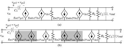
**Figure 5.5-7** (a) Small-signal model for Fig. 5.5-5(a). (b) Simplified small-signal model of (a).
