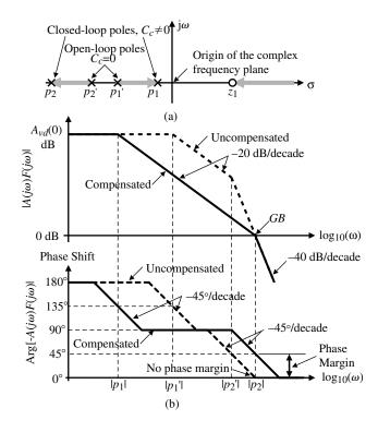
**Figure 6.2-7** (a) Root locus plot of the loop gain [F(s) = 1]resulting from the Miller compensation as  $C_C$  is varied from 0 to the value used to achieve the unprimed roots. (b) The asymptotic magnitude and phase plots of the loop gain [F(s) = 1]before and after compensation.
