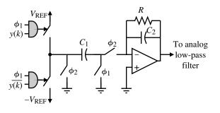
**Figure 9.9-18** A switched capacitor DAC implementation.
