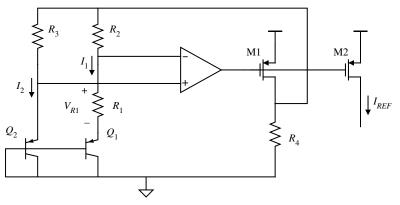
Figure P4.6-8 A temperature-independent reference current.
