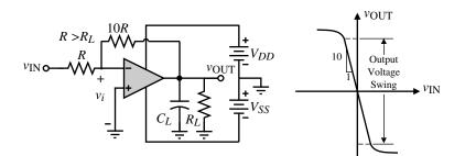
Figure 6.6-11 Measurement of the output-voltage swing.
