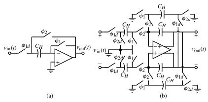
**Figure 9.5-12** (a) Switched capacitor S/H circuit that autozeroes the op amp inputoffset voltage. (b) A differential S/H that avoids large changes at the op amp output.
