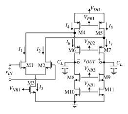
**Figure 7.3-6** Folded-cascode, differential-output op amp.
