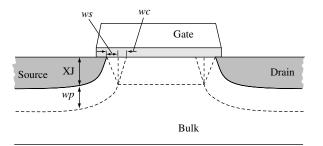
Figure 3.4-1 Illustration of the shortchannel effects in the MOS transistor.
