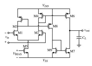
Figure 8.3-1 Clamped push–pull output comparator.
