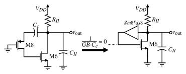
**Figure 6.2-17** Illustration of how the output pole is increased by Fig. 6.2-16(a).
