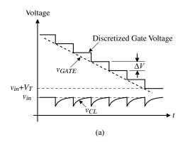
**Figure 4.1-10** Illustration of (a) slow ramp and (b) fast ramp using a quantized voltage ramp to illustrate the effects due to the time constant of the channel resistance and capacitance.
