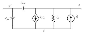
**Figure C.2-1** Small-signal MOS transistor model including noise current.
