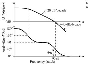
Figure 6.2-2 Frequency and phase response of a second-order system.
