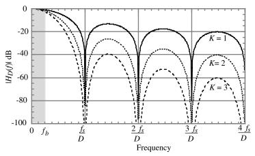
Figure 9.9-11 Magnitude response of a cascaded comb filter for K = 1, 2, and 3.
