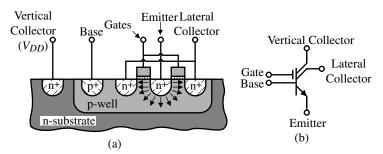
**Figure 7.5-4** (a) Cross section of a field-aided NPN lateral BJT. (b) Symbol for (a).
