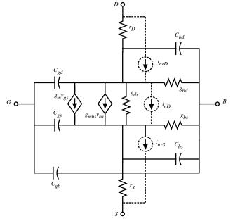
The conductances  $g_{bd}$  and  $g_{bs}$  are the equivalent conductances of the bulk-to-drain and bulk-to-source junctions. Since these junctions are normally reverse biased, the conductances are very small. They are defined as
