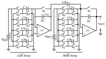
**Figure 9.3-6** Combination of two, 4-bit, binary-weighted, charge amplifier subDACs to form an 8-bit, binary-weighted, charge amplifier DAC.
