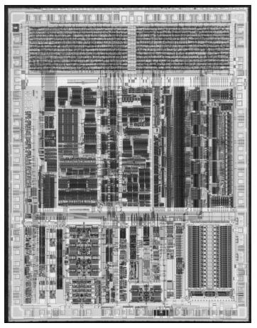
Figure 1.4-6 Photomicrograph of the read-channel chip.
