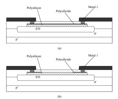
Figure 2.4-6 Polysilicon resistors: (a) without silicide block, (b) with silicide block.
