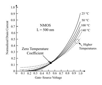
Figure 3.2-9 Zero temperature coefficient characteristics of a modern CMOS technology  $(L_{\min} = 50 \text{ nm}).$
