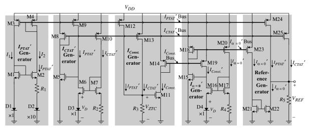
Figure 4.6-14 Transistor-level implementation of the low TC voltage reference in Fig. 4.6-13.
