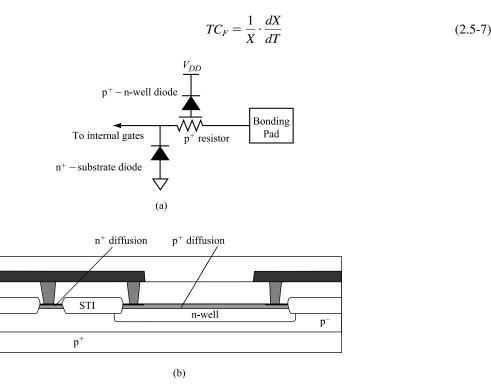
**Figure 2.5-5** Electrostatic discharge protection circuitry. (a) Electrical equivalent circuit. (b) Implementation in CMOS technology.
