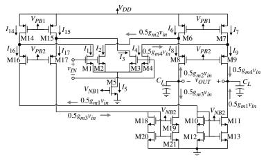
Figure 7.3-8 Class B, folded-cascode, differential-output op amp.
