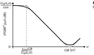
**Figure 6.4-3** Magnitude of the PSRR<sup>+</sup> for a two-stage op amp.
