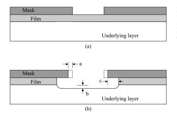
Figure 2.1-3 (a) Portion of the top layer ready for etching. (b) Result of etching indicating horizontal etching and etching of underlying layer.
