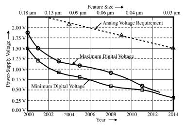
Figure 7.6-2 Roadmap for supply voltage for CMOS technology.
