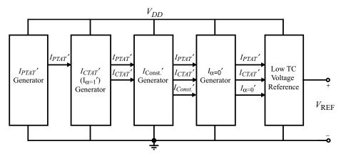
Figure 4.6-12 Block diagram of the parallel form of the curvature corrected temperature stable reference.
