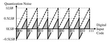
Figure 9.1-5 Quantization noise for the 3-bit DAC of Fig. 9.1-4.
