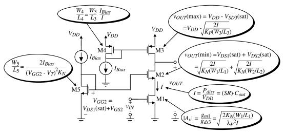
Figure 5.3-7 Pertinent design equations for the simple cascode amplifier of Fig. 5.3-1.
