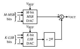
Figure 9.3-1 Combining an *M*-bit and *K*-bit subDAC to form an M + K-bit DAC by dividing the output of the *K*-*LSB* DAC.
