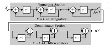
Figure 9.9-12 Implementation of a cascaded comb filter.
