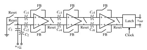
Figure 8.6-3 Fully differential, three-stage comparator and latch.
