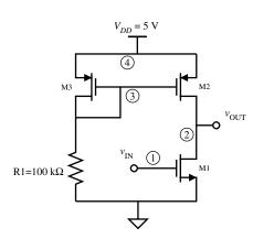
**Figure 3.6-4** A simple MOS amplifier for Example 3.6-2.
