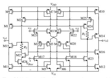
Figure 7.3-11 Class AB differential-output op amp using a cross-coupled differential-input stage.
