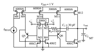
Figure 7.6-18 A 1 V, two-stage operational amplifier.
