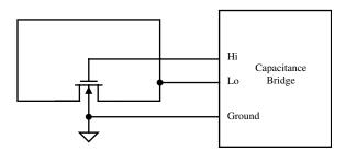
**Figure C.5-2** Experimental setup for measuring  $C_{GS}$  and  $C_{GD}$ .
