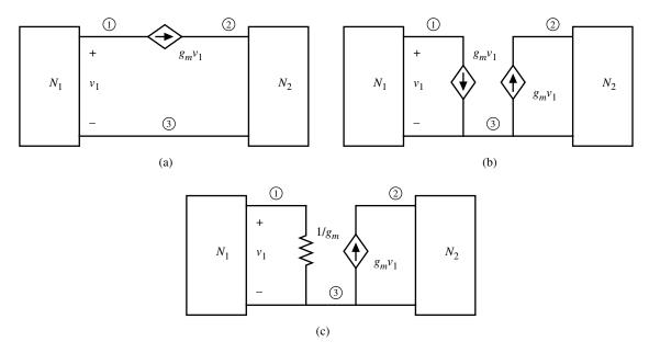
**Figure A.1-6** Current-source rearrangement and substitution. (a) Original circuit. (b) Rearrangement of current source. (c) Substitution of current source by a resistor  $1/g_m$ .
