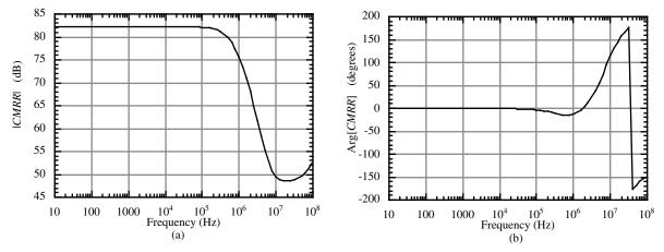
**Figure 6.6-8** CMRR frequency response of Example 6.3-1 with  $C_c = 10$  pF. (a) Magnitude response. (b) Phase response.
