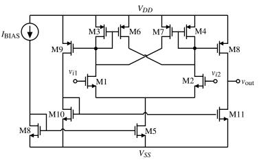
Figure 8.4-14 Complete comparator with internal hysteresis including an output stage.
