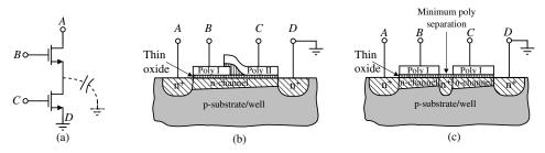
**Figure 6.5-7** (a) Cascode amplifier with parasitic capacitance. Method of reducing source/drainto-bulk capacitance for (b) a double poly technology and (c) a single poly technology.
