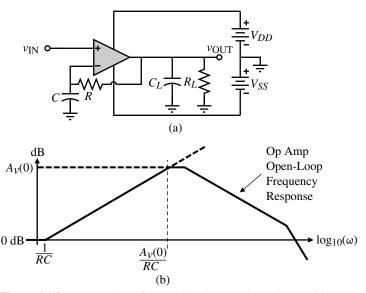
**Figure 6.6-2** (a) A method of measuring the open-loop characteristics with dc bias stability. (b) Asymptotic magnitude plot of the voltage-transfer function.
