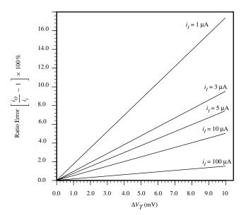
**Figure 4.4-3** Plot of ratio error (in %) versus offset voltage for the current mirror of Fig. 4.4-1. For this plot,  $v_{T1} = 0.7$  V and  $K'W/L = 110 \mu A/V^2$ .
