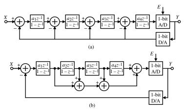
**Figure 9.9-8** (a) A fourth-order distributed feedback modulator. (b) A fourth-order distributed feedforward modulator.
