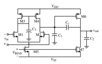
**Figure 6.2-8** A two-stage op amp with various parasitic and circuit capacitances shown.
