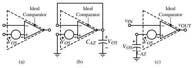
**Figure 8.4-1** (a) Simple model of a comparator including offset. (b) Comparator in unity-gain configuration storing the offset on autozero capacitor  $C_{AZ}$  during the first half of the autozero cycle. (c) Comparator in open-loop configuration with offset cancellation achieved at the noninverting input during the second half of the autozero cycle.
