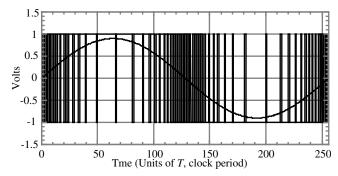
Figure 9.9-4 First-order modulator output for a sinusoidal input.
