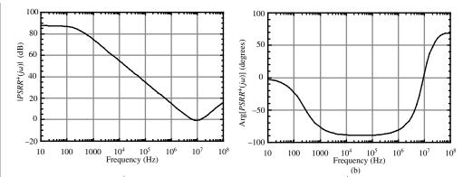
**Figure 6.6-18** (a) PSRR<sup>+</sup> magnitude response of Example 6.6-1. (b) PSRR<sup>+</sup> phase response of Example 6.6-1.
