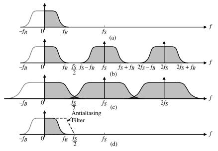
**Figure 9.5-2** (a) Continuous time frequency response of the analog input signal. (b) Sampled-data equivalent frequency response. (c) Case where  $f_B$  is larger than  $0.5f_S$ , causing aliasing. (d) Use of an antialiasing filter to avoid aliasing.
