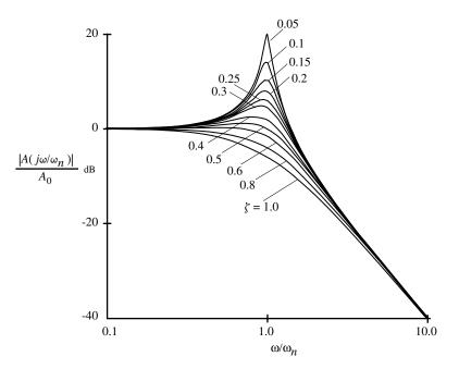
Figure D.1-2 Gain magnitude response for various values of  $\zeta$  for a second-order, low-pass system.
