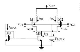
**Figure 5.2-2** CMOS differential amplifier using NMOS transistors.
