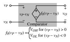
Figure 8.1-3 Model for an ideal comparator.
