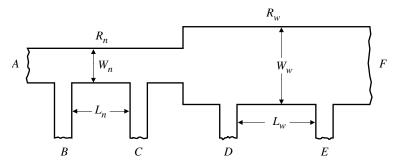
Figure C.4-1 Sheet resistance and bias monitor.
