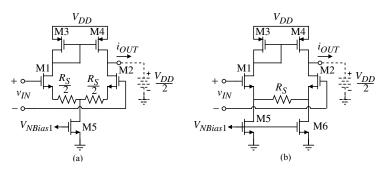
Figure 5.2-18 Two different ways of degenerating the differential amplifier.
