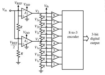
**Figure 9.8-3** A 3-bit interpolating ADC with an interpolation factor of 4.
