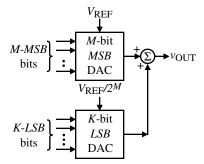
**Figure 9.3-2** Combining an *M*-bit and *K*-bit subDAC to form an M + K-bit DAC by dividing the  $V_{\text{REF}}$  to the *K*-*LSB* DAC (subranging).
