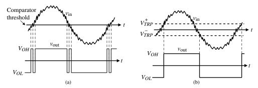
Figure 8.4-6 (a) Comparator response to a noisy input. (b) Comparator response to a noisy input when hysteresis is added.
