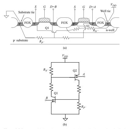
**Figure 2.5-3** (a) Parasitic lateral NPN and vertical PNP bipolar transistor in CMOS integrated circuits. (b) Equivalent circuit of the SCR formed from the parasitic bipolar transistors.
