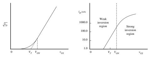
Figure 3.5-1 Weak inversion characteristics of the MOS transistor as modeled by Eq. (3.5-4).
