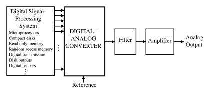
Figure 9.1-1 Digital-analog converter in signal-processing applications.
