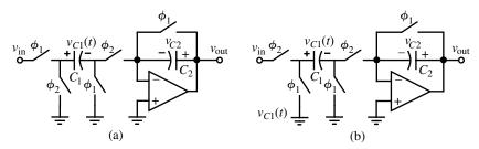
**Figure E.2-7** (a) Noninverting and (b) inverting switched capacitor voltage amplifiers that are insensitive to parasitic capacitors.
