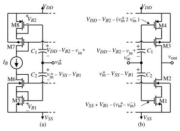
**Figure 7.2-6** (a) Equivalent circuit for Fig. 7.2-5 during the  $\phi_1$  clock period. (b) Equivalent circuit for Fig. 7.2-5 during the  $\phi_2$  clock period.
