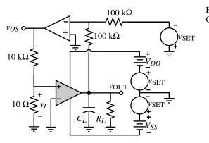
**Figure 6.6-6** Circuit used to measure CMMR and PSRR.
