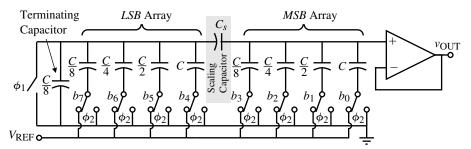
Figure 9.3-4 Combination of two, 4-bit charge scaling subDACs to form an 8-bit charge scaling DAC.
