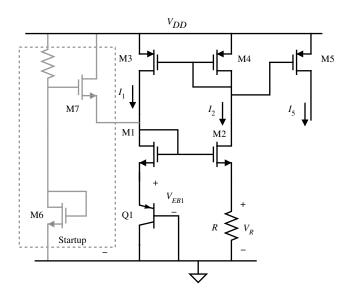
Figure 4.5-6 Base–emitter voltage-referenced circuit.
