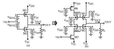
**Figure 5.5-5** (a) Push–pull, source follower. (b) Push–pull, source follower showing the implementation of the floating batteries,  $V_{\text{BIAS}}$ .
