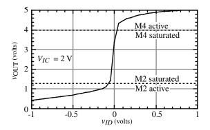
**Figure 5.2-7** Voltage-transfer curve for the differential amplifier of Fig. 5.2-6.
