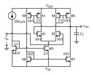
**Figure 7.1-9** Simple shunt negative-feedback buffer.
