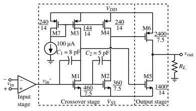
Figure 7.1-2 A CMOS op amp with low-impedance drive capability.
