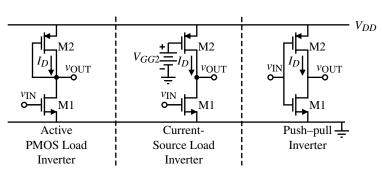
Figure 5.1-1 Various types of inverting CMOS amplifiers.
