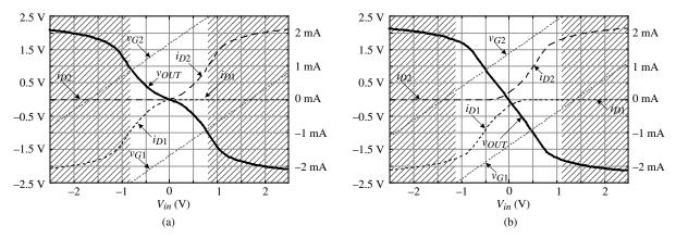
**Figure 5.5-10** Output voltage and current characteristics for the push–pull, common-source amplifier of Fig. 5.5-8 for (a) Class B and (b) Class AB operation. Operation in the shaded areas is not possible unless  $V_{in}$  can be outside the rails.
