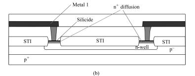
Figure 2.4-5 Resistors: (a) diffusion, (b) n-well.
