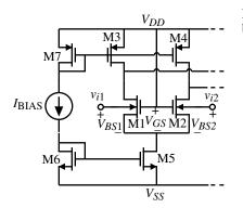
**Figure 7.6-10** Low-voltage differential input using bulk–source-driven input transistors.
