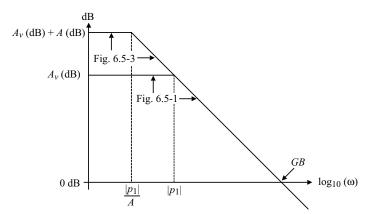
Figure 6.5-4 Comparison of the frequency response of Figs. 6.5-1 and 6.5-3.
