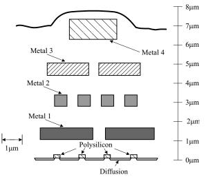
Figure 2.1-6 Side view of a CMOS integrated circuit.
