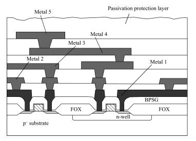
Figure 2.1-8 Cross section of a LOCOS CMOS process.
