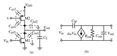
**Figure 5.1-4** (a) General configuration of an inverter illustrating the parasitic capacitances. (b) Small-signal model of (a).
