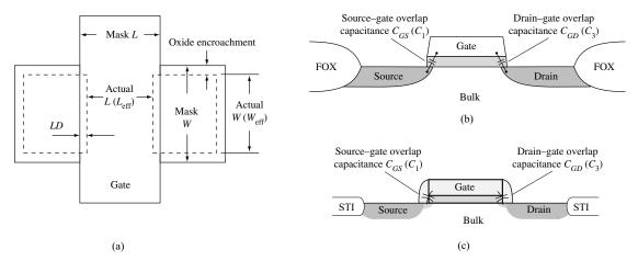
Figure 3.2-5 Overlap capacitances of an MOS transistor. (a) Top view showing the overlap between the source or drain and the gate for LOCOS technology. (b) Side view for LOCOS technology. (c) Side view for STI technology.
