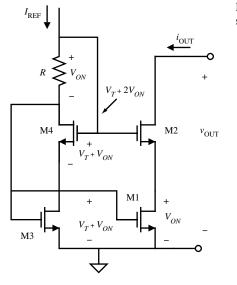
The back-gate bias on M2 and M4 is -0.25 V. Therefore, the threshold voltage for M2 and M4 is calculated to be
