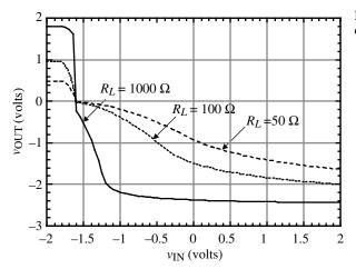
**Figure 7.1-14** Influence of  $R_L$  on the output voltage of Fig. 7.1-12.
