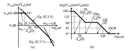
**Figure E.3-3** (a) Magnitude and (b) phase response of a continuous time inverting integrator when  $A_{vd}(0)$  and *GB* are finite.
