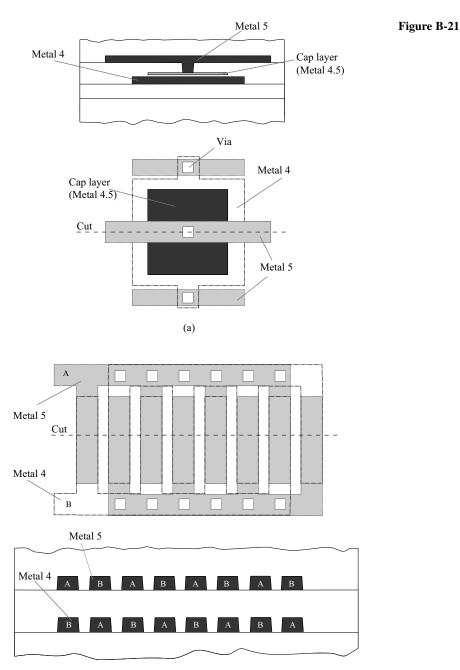
oxide thickness. If the error is caused by a uniform linear variation in the oxide thickness, then a common-centroid geometry can be used to eliminate its effects [2]. Area-related errors result from the inability to precisely define the dimensions of the capacitor on the integrated circuit. This is due to the error tolerance associated with making the mask, the nonuniform etching of the material defining the capacitor plates, and other limitations [3].
