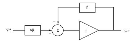
Figure D.1-3 Single-loop feedback block diagram.
