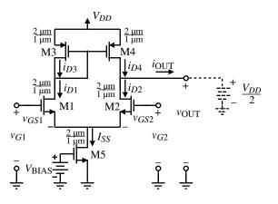
**Figure 5.2-6** CMOS differential amplifier using a current-mirror load.
