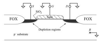
Figure 2.3-2 Cross section of an n-channel transistor with all terminals grounded.
