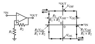
Figure 8.4-8 Inverting bistable circuit using external positive feedback.
