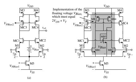
**Figure 6.5-1** (a) Cascoding of the first stage of the two-stage op amp. (b) Implementation of the floating voltage,  $V_{Bias}$ .
