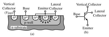
Figure 7.5-3 (a) Cross section of an NPN lateral BJT. (b) Symbol for (a).
