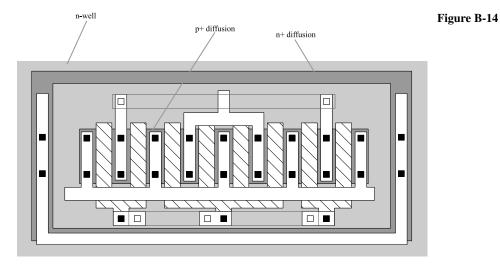
remedied by encircling the matched devices with a well tie as illustrated in Fig. B-14. In this example, the transistor array is surrounded by a well tie.
