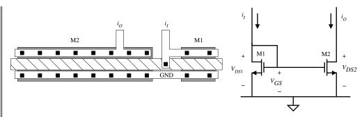
**Figure 4.4-4** Layout of current mirror without  $\Delta W$  correction.
