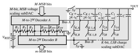
Figure 9.3-7 M + K-bit DAC using an M-bit voltage scaling subDAC for the MSBs and a K-bit charge scaling subDAC for the LSBs.
