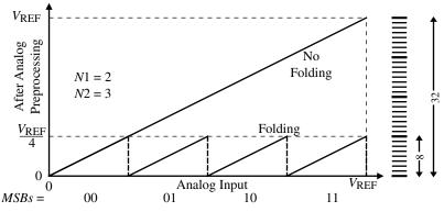
Figure 9.8-9 Folding characteristic for N1 = 2 and N2 = 3.
