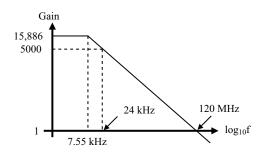
Figure 9.5-20 Magnitude response of the sample-and-hold on amp.
