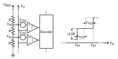
Figure 9.8-2 Flash ADC for Example 9.8-1.
