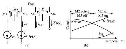
**Figure 7.6-16** (a) Circuit to generate nonlinear correction term,  $I_{\rm NL}$ . (b) Illustration of the various currents in (a).
