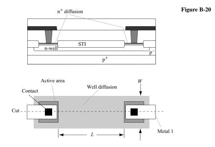
area near the transitions under the contact region. It is convenient to measure L and W as shown and then characterize the total resistance in two components: the body component of the resistor (the portion along the length, L) and the contact component. One could choose a different approach as long as devices are characterized consistently with the measurement.
