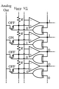
Figure 9.8-16 Implementation of the DAC in the pipeline stage.
