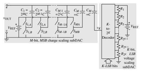
Figure 9.3-9 M + K-bit DAC using an M-bit charge scaling subDAC for the MSBs and a K-bit voltage scaling subDAC for the LSBs.
