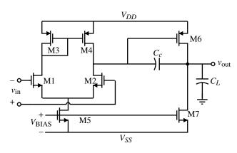
**Figure 7.4-1** Two-stage Miller op amp operating in weak inversion.
