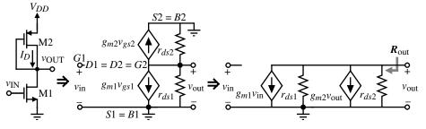
**Figure 5.1-3** Development of the small-signal model for the active load inverter.
