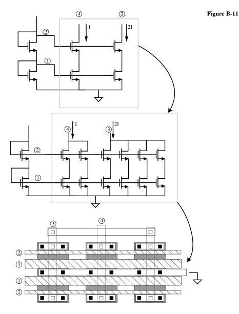
(common node where source and drain connect) of one unit pair is not electrically connected to the other unit pair. There are strategies to avoid drawing the extra transistors but these are specific to the CAD (computer-aided design) software being used and the methodology chosen.
