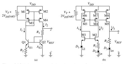
**Figure 4.6-8** Series temperature-independent voltage references using (a) MOSFETs and BJTs and (b) only MOSFETs and diodes.
