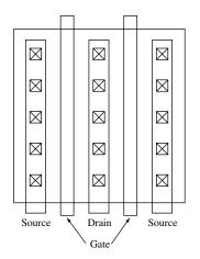
Figure C.5-1 Structure for determining  $C_{GS}$  and  $C_{GD}$ .
