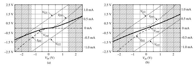
Figure 5.5-6 Output voltage and current characteristics for the push–pull, source follower of Fig. 5.5-5(a) for (a) Class B and (b) Class AB operation. Operation in the shaded areas is not possible unless  $V_{in}$  can be outside the rails.
