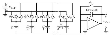
Figure 9.2-12 Binary-weighted, charge amplifier DAC implementation.
