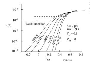
**Figure 3.5-3** Transfer characteristics of a long-channel device as a function of temperature. (Copyright © 1977).
