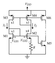
Figure 4.5-7 Simple, power-supply independent current reference.
