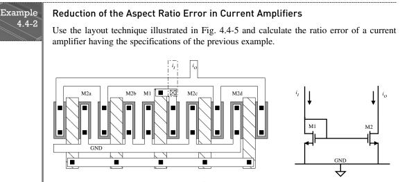
Figure 4.4-5 Layout of current mirror with  $\Delta W$  correction as well as common-centroid layout techniques.
