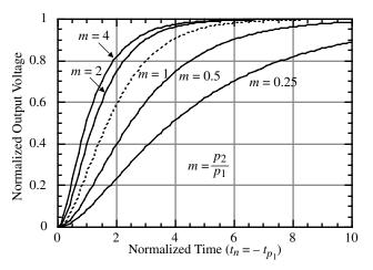
**Figure 8.2-2** Linear step response of a comparator with two real axis poles,  $p_1$  and  $p_2$ .
