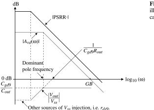
Figure 6.5-13 Approximate graphical illustration of the PSRR<sup>-</sup> for the folded-cascode op amp.
