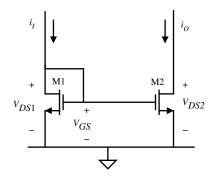
Consequently,  $i_O/i_I$  is a function of the aspect ratios that are under the control of the designer.
