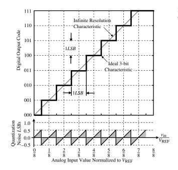
Figure 9.5-3 Ideal input–output characteristics of a 3-bit ADC.
