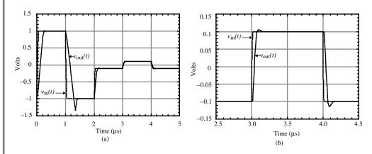
**Figure 6.6-20** (a) Unity-gain transient response of Example 6.6-1. (b) Unity-gain, small-signal transient response of Example 6.6-1.
