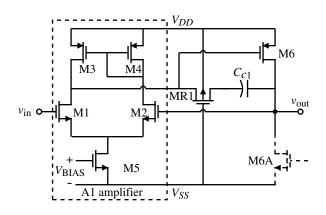
**Figure 7.1-7** Positive output stage, unity-gain amplifier.
