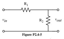
2.4-6. Repeat Problem 2.4-5 using a  $n^+$  diffused resistor for  $R_1$ . Assume that a  $n^+$  resistor's voltage coefficient is 200 ppm/V.
