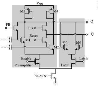
Figure 8.6-4 Example of a preamplifier and latch.
