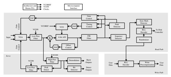
Figure 1.4-1 Read/Write channel integrated-circuit block diagram.
