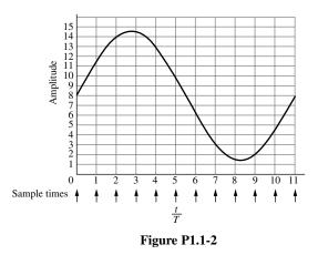
1.1-3. Digitize the sinusoid given in Fig. P1.1-2 according to Eq. (1.1-1) using a 4-bit digitizer.
