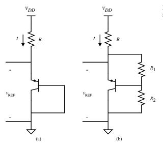
**Figure 4.5-3** (a) pn Junction voltage reference. (b) Increasing  $V_{\text{REF}}$  of (a).
