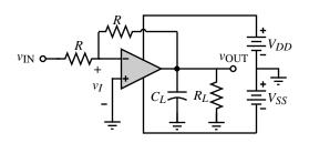
**Figure 6.6-3** Configuration for simulating or measuring the open-loop frequency response for moderate-gain op amps.
