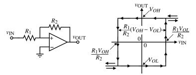
Figure 8.4-7 Noninverting bistable circuit using external positive feedback.
