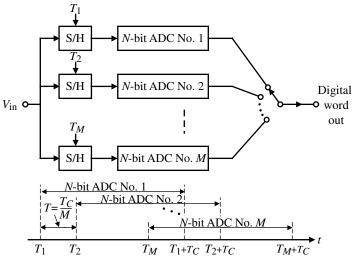
Figure 9.8-20 A time-interleaved ADC.
