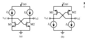
**Figure 8.5-3** (a) NMOS latch. (b) PMOS latch.
