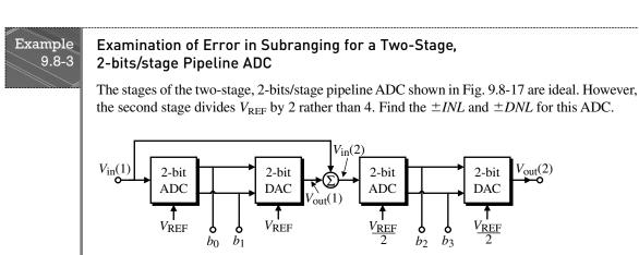
Figure 9.8-17 Pipeline ADC for Example 9.8-3.
