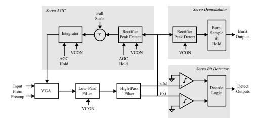
Figure 1.4-5 Servo channel block diagram.
