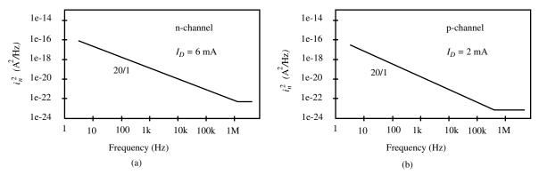
Figure 3.2-8 Drain-current noise for (a) an n-channel and (b) a p-channel MOSFET measured on a silicon-gate submicron process.
