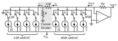
Figure 9.3-3 Combination of current scaling subDACs using a current divider.
