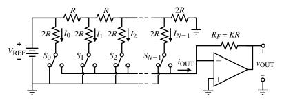
Figure 9.2-4 *R*–2*R* ladder implementation of the binary-weighted resistor DAC.
