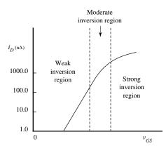
**Figure 3.5-2** The three regions of operation of an MOS transistor.
