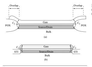
**Figure 3.2-6** Gate–bulk overlap capacitances. (a) LOCOS technology. (b) STI technology.
