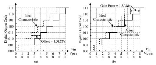
Figure 9.5-4 (a) Example of offset error for a 3-bit ADC. (b) Example of gain error for a 3-bit ADC.
