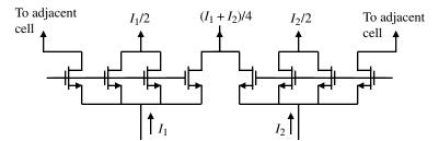
Figure 9.8-5 Current (active) interpolation using current mirrors.
