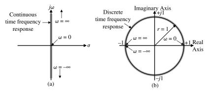
Figure E.1-7 (a) Continuous frequency domain. (b) Discrete frequency domain.
