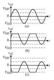
**Figure 7.3-2** Influence of the common-mode (CM) signal on the differential-mode signal. (a) CM = 0. (b)  $CM = 0.5V_{DD}$ . (c)  $CM = 0.5V_{SS}$ .
