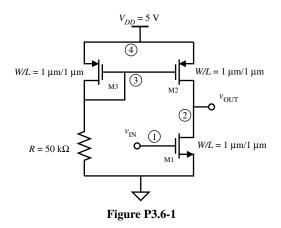
**3.6-2.** Use SPICE to perform the following analyses on the circuit shown in Fig. P3.6-1: (a) Plot  $v_{OUT}$  versus  $v_{IN}$  for the nominal parameter set shown. (b) Separately, vary K' and  $V_T$  by +10% and repeat part (a)—four simulations.
