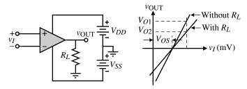
Figure 6.6-12 Measurement of the open-loop output resistance.
