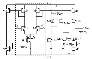
**Figure 7.4-3** Op amp of Fig. 7.4-2 using cascode outputs for gain improvement in weak inversion operation.
