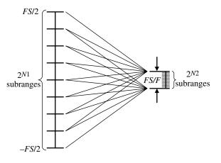
Figure 9.8-8 Illustration of the folding concept.
