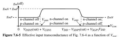
Figure 7.6-5 Effective input transconductance of Fig. 7.6-4 as a function of  $V_{icm}$ .
