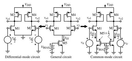
**Figure 5.2-10** Illustration of the simplications of the differential amplifier for small-signal, differential-mode, and common-mode analysis.
