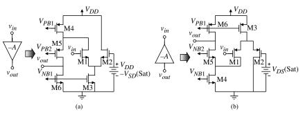
**Figure 6.5-15** Enhancement amplifier realizations for (a) the upper amplifier and (b) the lower amplifier.
