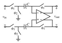
Figure 8.5-2 A differential-in, differential-out, switched capacitor comparator.
