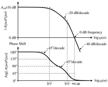
**Figure 6.2-5** The open-loop frequency response of a negative-feedback loop using an uncompensated op amp and a feedback factor of F(s) = 1.
