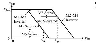
Figure 7.1-3 Idealized voltage-transfer characteristic of the crossover inverters.
