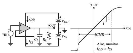
Figure 6.6-10 Measurement of the input common-mode voltage range of an op amp.
