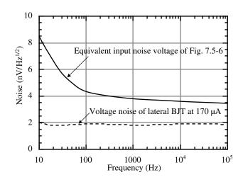
**Figure 7.5-7** Experimental noise performance of Fig. 7.5-6.
