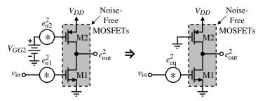
Figure 5.1-12 Noise calculations in a current-source load inverter.
