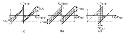
Figure 9.7-12 (a) Gain error,  $A_i$ . (b) System offset error,  $V_{OSi}$ . (c) Comparator offset error,  $V_{OCi}$ .
