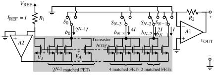
Figure 9.2-5 Current scaling using matched MOSFETs.
