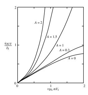
**Figure 7.4-5** Parametric curves showing normalized output current versus input voltage for different values of *A*.
