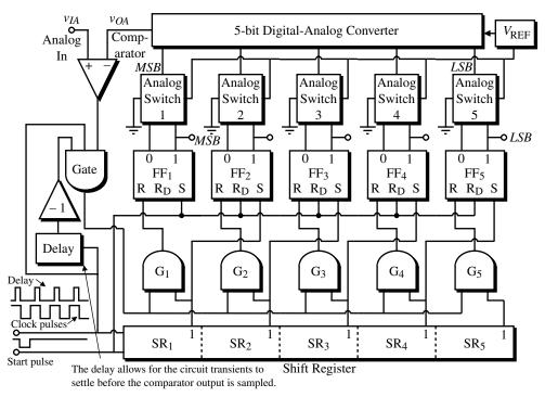
Figure 9.7-3 A 5-bit successive-approximation ADC with shift register control. (From E. R. Hnatek, *A User's Handbook of D/A and A/D Converters*. New York: Wiley, 1976.)
