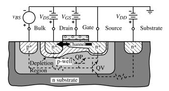
Figure 7.6-8 Cross section of an n-channel bulk-driven MOSFET.
