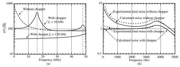
**Figure 7.5-11** (a) Experimentally observed op amp equivalent input noise for various chopping frequencies. (b) Experimentally observed filter output noise with and without chopper, compared to theoretically predicted total noise.
