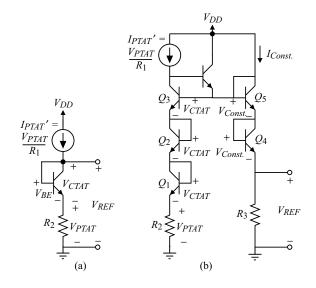
**Figure 4.6-11** (a) Series temperatureindependent voltage reference. (b) Method of correcting for the bandgap curvature problem. As before, if we assume that the current density,  $J_D$ , in Eq. (4.6-14) has a temperature dependence of  $T^{\alpha}$ , then we can rewrite Eq. (4.6-14) as
