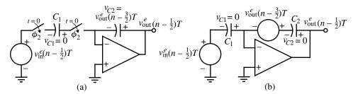
**Figure E.3-7** (a) Equivalent circuit of Fig. E.3-4(b) at the moment the  $\phi_2$  switches close. (b) Simplified equivalent circuit of (a).
