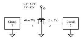
Figure 4.1-5 Application of an n-channel transistor as a switch with typical terminal voltages indicated.
