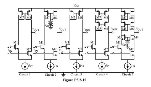
equivalent-input-noise voltage for this amplifier if  $W_1/L_1 = W_2/L_2 = 2 \ \mu m/1 \ \mu m$ ,  $W_3/L_3 = W_4/L_4 = 1 \ \mu m/1 \ \mu m$ , and  $I_{SS} = 50 \ \mu A$ . What is the equivalent-output-noise current under these conditions?
