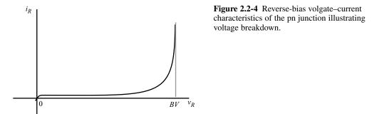
Zener breakdown, which generally occurs at voltages less than 6 volts. Zener diodes can be fabricated where an  $n^+$  diffusion overlaps with a  $p^+$  diffusion. Note that the Zener diode is compatible with the basic CMOS process although one terminal of the Zener must be either on the lowest power supply, ground, or the highest power supply,  $V_{DD}$ .
