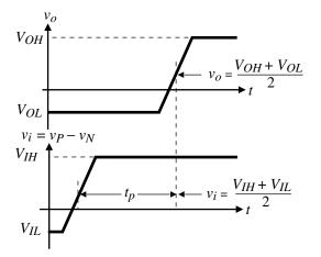
**Figure 8.1-9** Propagation delay time of a noninverting comparator.
