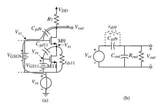
**Figure 6.5-12** (a) Portion of Fig. 6.5-9(b) used to examine PSRR<sup>-</sup>. (b) Model of (a).
