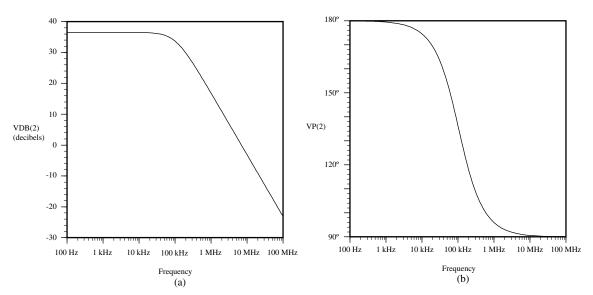
Figure 3.6-6 (a) Magnitude response and (b) phase response of Example 3.6-3.
