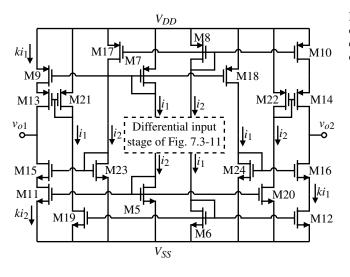
**Figure 7.4-7** Implementation of the current-mirror boosting concept using the differential-output op amp of Fig. 7.3-11.
