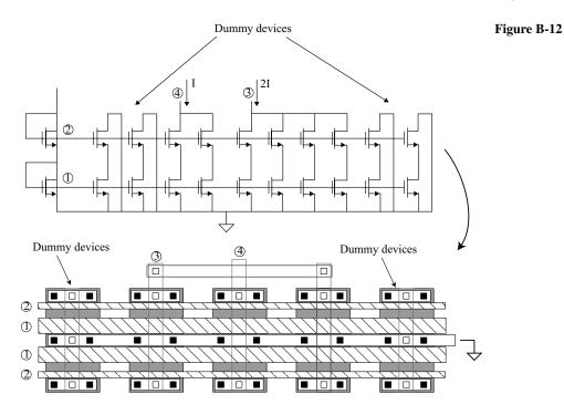
transistors at either side do not see other similar transistors. Thus, one of the fundamental matching principles has been violated. This is easily solved by adding transistors that have no electrical function but serve to achieve the "same periphery" matching principle. Figure B-12 is a modification of Fig. B-11 with the addition of "dummy" transistors.
