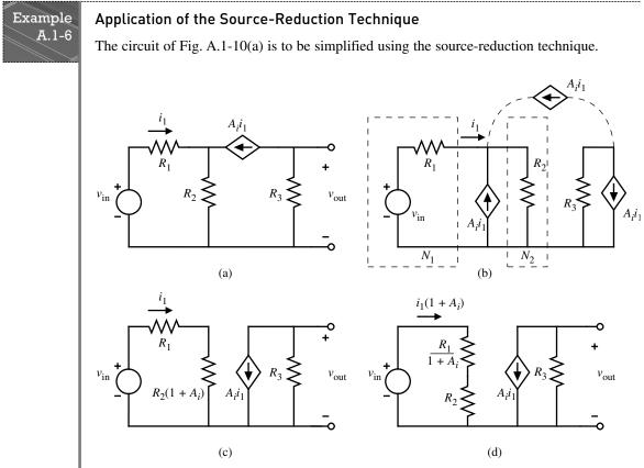
**Figure A.1-10** Current reduction. (a) Original circuit. (b) Identification of  $N_1$  and  $N_2$ . (c) Modification of  $N_2$ . (d) Modification of  $N_1$ .
