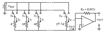
Figure 9.2-3 Binary-weighted resistor DAC implementation.
