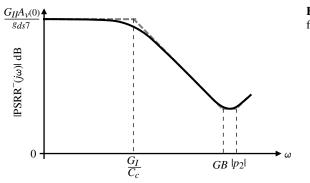
**Figure 6.4-5** Magnitude of the PSRR<sup>-</sup> for a two-stage op amp.
