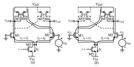
**Figure 8.4-12** (a) Comparator of Fig. 8.4-11 where  $v_{in}$  is very negative and increasing toward  $V_{TRP}^+$  (b) Comparator of Fig. 8.4-11 where  $v_{in}$  is very positive and decreasing toward  $V_{TRP}^-$ .
