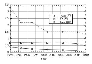
**Figure 7.6-1** Projection for CMOS technology.
