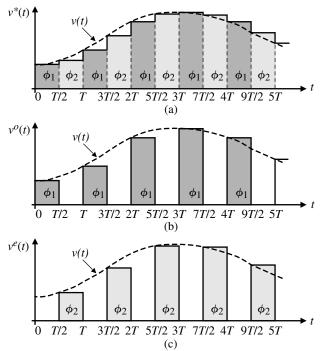
**Figure E.1-1** (a) A sampled-data voltage waveform for a two-phase clock. (b) Waveform for the odd clock ( $\phi_1$ ). (c) Waveform for the even clock ( $\phi_2$ ).
