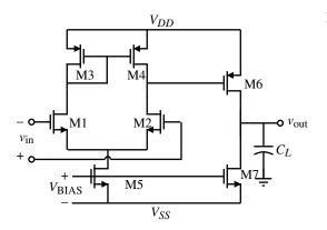
Figure 8.2-1 Two-stage comparator.
