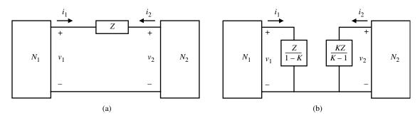
Figure A.1-11 Miller simplification. (a) Original circuit. (b) Equivalent circuit of (a).
