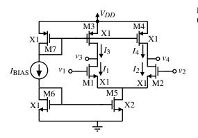
**Figure 5.2-14** A current-source load, differential amplifier.
