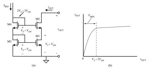
Figure 4.3-5 (a) Standard cascode current sink. (b) Output characteristics of circuit in (a).
