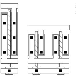
Figure 3.6-1 (a) M1 3 2 1 0 NCH W = 20U L = 1U.(b) M1 3 2 1 0 NCH W = 10U L = 1U M = 2. A SPICE simulation file for an MOS circuit is incomplete without a description of the model to be used to characterize the MOS transistors used in the circuit. A model is described by placing a line in the simulation file using the following format:
