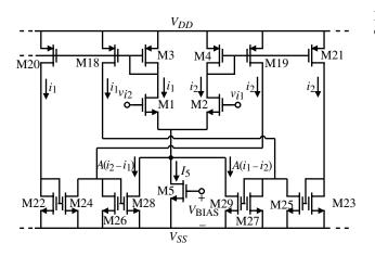
**Figure 7.4-4** Dynamically biased differential amplifier input stage.
