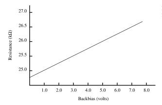
**Figure C.4-4** n-Well resistance as a function of backbias voltage.
