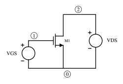
Figure 3.6-2 Circuit for Example 3.6-1.
