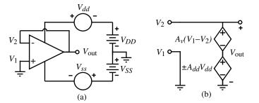
Figure 6.4-1 (a) Method for calculating PSRR. (b) Model (a).
