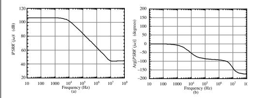
**Figure 6.6-19** (a) PSRR<sup>-</sup> magnitude response of Example 6.6-1. (b) PSRR<sup>-</sup> phase response of Example 6.6-1.
