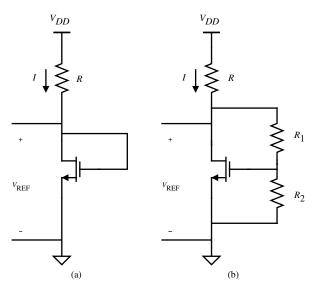
**Figure 4.5-4** (a) MOS equivalent of the pn junction voltage reference. (b) Increasing  $V_{\text{REF}}$  of (a).
