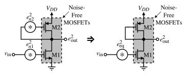
Figure 5.1-10 Noise calculations in an active load inverter.
