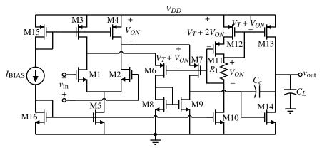
**Figure 7.6-17** A low-voltage, two-stage op amp having  $V_{DD} \ge V_T$ .
