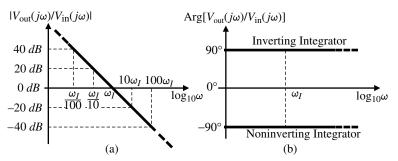
Figure E.3-2 (a) Ideal magnitude and (b) phase response for a noninverting and continuous time integrator.
