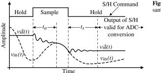
**Figure 9.5-7** Waveforms for a sample-and-hold circuit.
