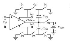
Figure 7.3-17 An external-output, common-mode voltage stabilization scheme.
