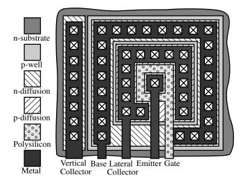
**Figure 7.5-5** Geometry of a lateral NPN transistor.
