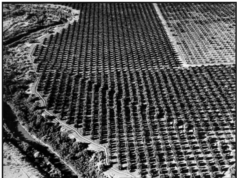
FIGURE 14.1 Fault displacement that occurred though an orange grove during an earthquake in Imperial Valley, California, in September, 1950. Photograph by David Scherman, Life Magazine © Time Inc.
