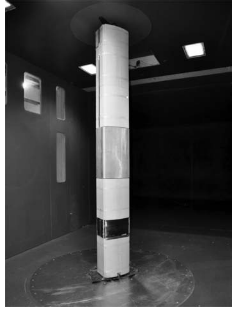
Figure 15. Cable stayed bridge tower sectional model in the wind tunnel test section: measure of static aerodynamic coefficients.
