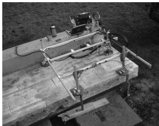
Figure 1. Automatic US-testing of the test specimen.
