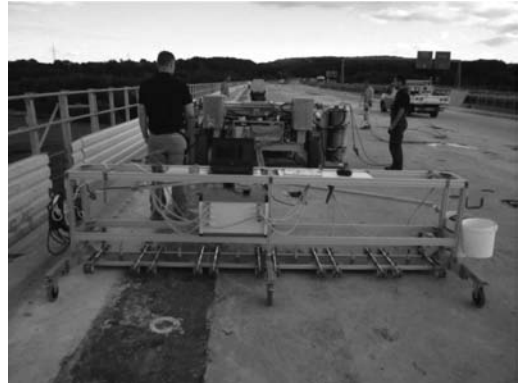
Figure 2. In-situ measurements with the large magnet and the newly developed line scanner on a highway bridge in Germany.
