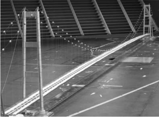
Figure 17. Full aeroelastic model on the turning table of Polimi Wind Tunnel. Length of the model 14 m.
