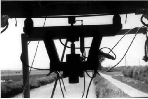
Figure 7. Measurement of the tension of a prestressing wire by the crossbow method.
