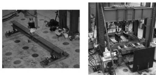
Figure 1. Set-up of fatigue tests on transverse stiffeners and horizontally lying shear studs.
