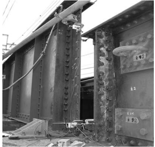
Figure 3. Sensors installed at girder ends.
