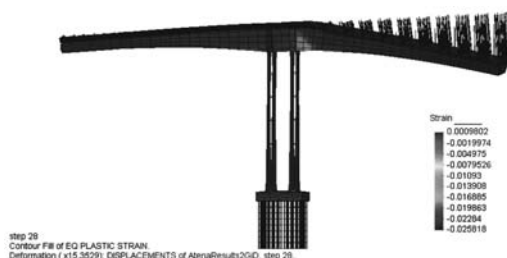
Figure 2. Plastic hinge formation at ultimate limit state.
