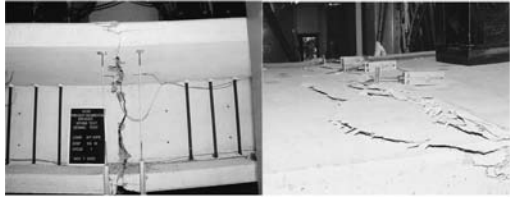
(c) Joint J3 at Failure in Unit 100-INT-AUX
