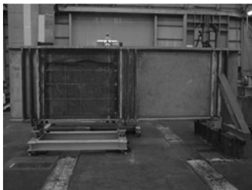
Figure 2. Specimen of corroded plate girder.
