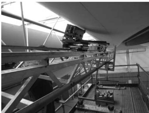
Figure 1. Magnet-Sensor-Unit, which was adapted by a substructure at the curvature of the double-curved HP-shells.
