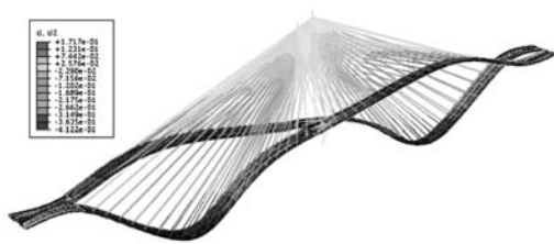
Figure 2. Deformations of the bridge under 40 trucks (scheme S3).
