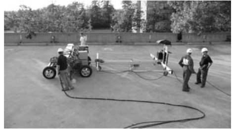
Figure 2. Detecting fractures in pre-stressing tendons on a parking deck with the big magnetic testing device.
