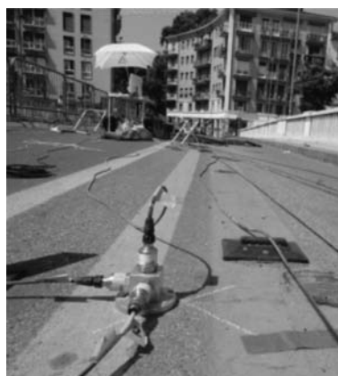
Figure 3. Setup scheme, a typical 3-axes accelerometer.
