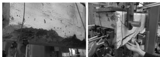
Figure 1. Severely corroded test specimen with cover spalling; before testing and at failure.
