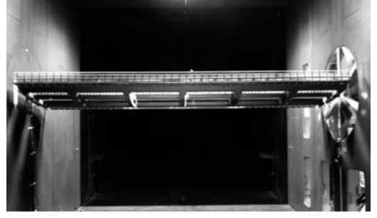
Figure 4. Deck sectional model in wind tunnel (external balance).
