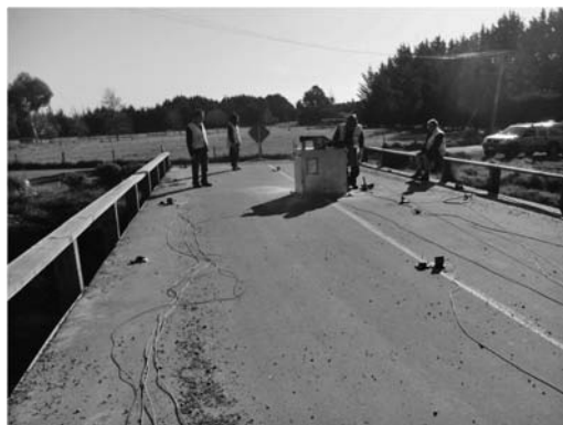
Figure 1. Setup of shaker and accelerometers for forced vibration tests.
