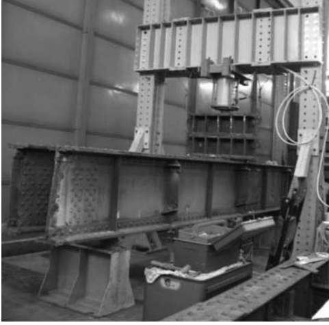
Figure 4. Bending tests on the structural elements taken for the railway bridge at the University of Padova.
