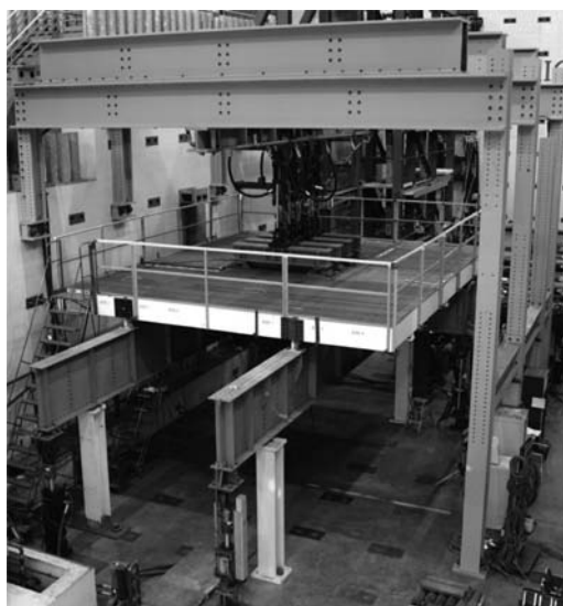
Figure 1. Full scale laboratory testing of orthotropic deck.
