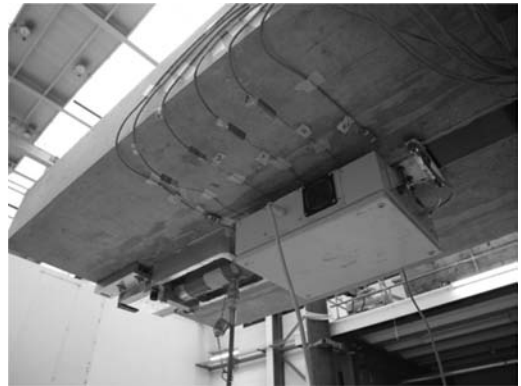
Figure 1. Prestressing and heating device for the gradient anchorage installation.
