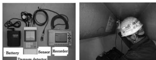
Photo 2. The non-destructive inspection of orthotropic steel deck.
