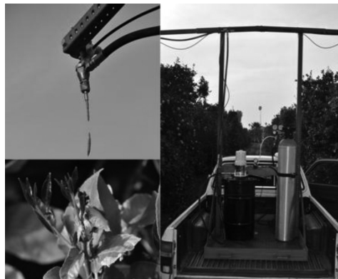
Figure 16.2 Mechanical application of SPLAT. Here, SPLAT is dispensed from a 57-L drum using a pneumatic pump supplied by an air tank (alternatively, a gas-powered air compressor may be used). This basic model can be replicated in any number of ways depending on the equipment available and field characteristics.
