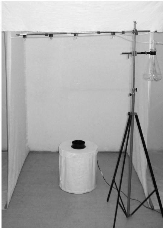
Figure 6.5 Room test setup with repellent-dispensing system and BG-Sentinel trap. (From Obermayr et al., J. Med. Entomol. , 49 (6), 1387, 2012.)
