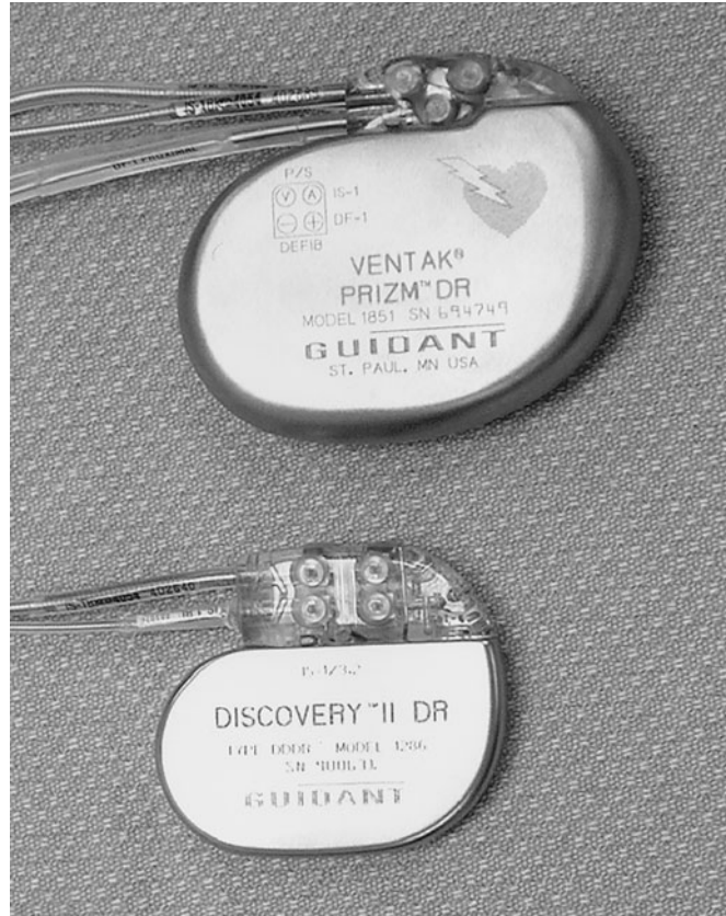
FIGURE 3.8 The generators of a modern cardioverter-defibrillator (Ventak Prizm DR, Guidant Corporation, Minneapolis, MN) and pacemaker (Discovery II DR, Guidant Corporation, Minneapolis, MN) are shown in the figure. Both are dual chamber devices, with the cardioverter-defibrillator possessing pacing features in addition to the core cardioversion hardware. The added hardware and power requirements demand a larger housing for this device in comparison to the pacemaker.
