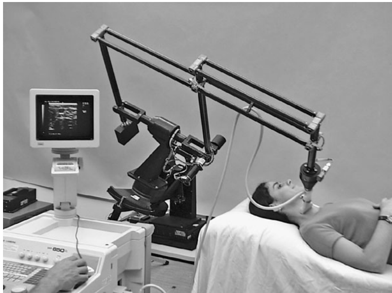
FIGURE 14.10 Robotic system for diagnostic ultrasound. 148 (Photo courtesy S. Salcudean.)
