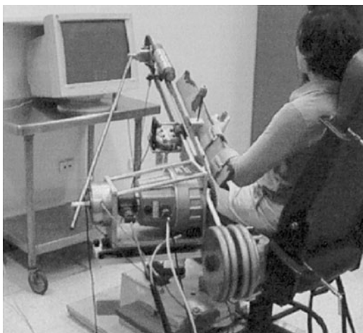
FIGURE 19.3 The ARM Guide. The patient's arm is attached to a hand splint (S) that is attached to an orientable linear track. A dc servo motor (M) can assist in movement of the subject's arm in the reaching direction (R) along the linear track. Optical encoders record position in the reach (R), pitch (P), and yaw (Y) axes. A six-axis force sensor (F) records the forces and torques at the interface between the device and the subject. The device is statically counterbalanced with two counterbalance weights (C).
