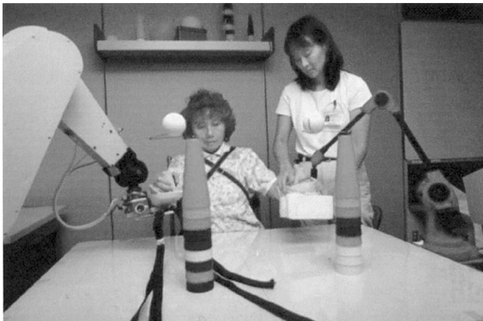
FIGURE 19.2 MIMe rehabilitator being used in bimanual mode. When the patient moves her unimpaired arm (left arm), a mechanical digitizing stylus senses the movement. The PUMA 560 robot arm then moves the patient's impaired arm (right arm) along a mirror-symmetrical trajectory. (From C. G. Burgar, P. S. Lum, P. C. Shor, and H. F. M. Van der Loos, Development of robots for rehabilitation therapy: The Palo Alto VA/Stanford experience , Journal of Rehabilitation Research and Development 37:663–673, 2000. Used with permission.)
