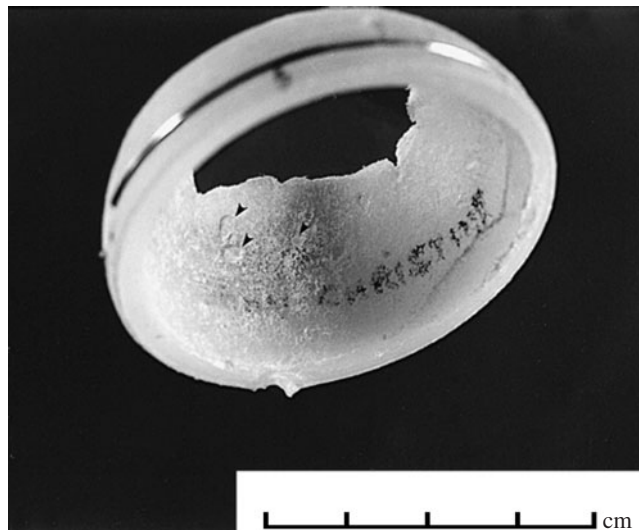
FIGURE 22.2 A cemented acetabular implant revised for aseptic loosening. Severe wear is associated with three-body abrasion caused by cement particles found at the articulating interface. (Printed with permission from Ref. 27.)
