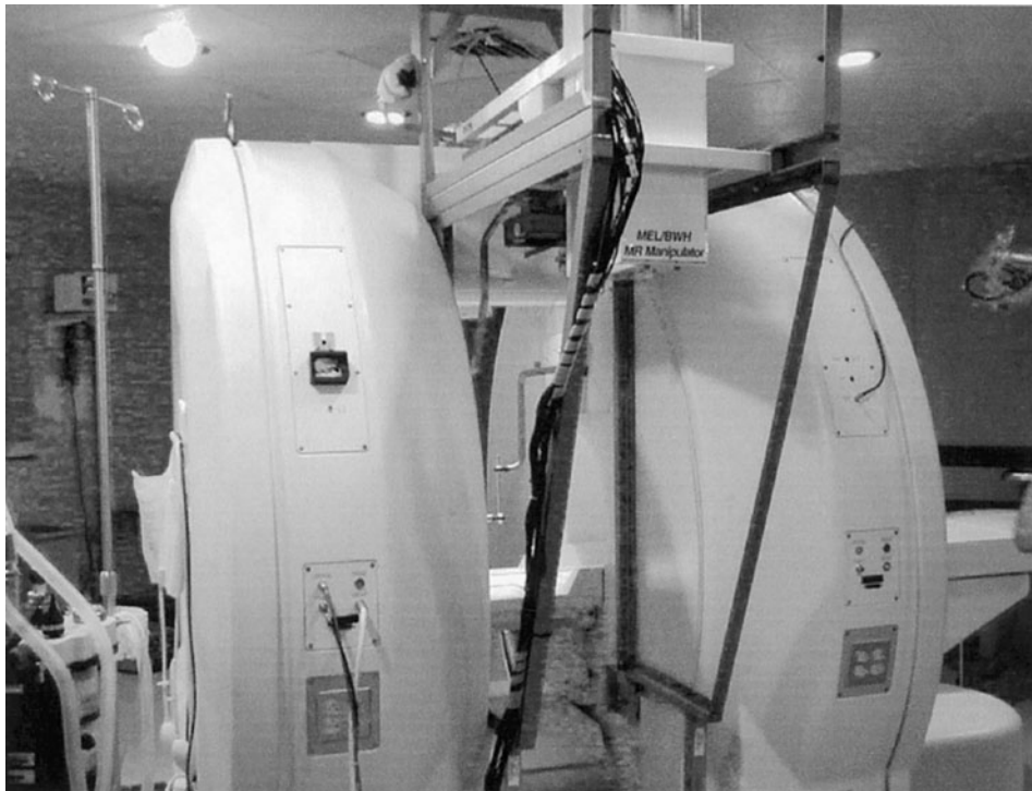
FIGURE 14.13 Robot system for use in open-magnet MRI system. 117
