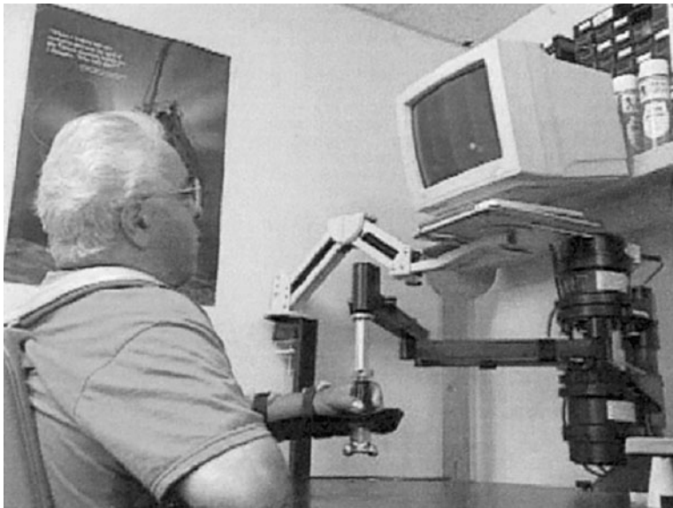
FIGURE 19.1 MIT-MANUS. (a) The patient attaches to the robot through a splint. The patient can move the robot or the robot can move the patient in the horizontal plane. The patient receives feedback of the hand trajectory on the computer screen. (From H. I. Krebs, B. T. Volpe, M. L. Aisen, and N. Hogan, Increasing productivity and quality of care: Robot-aided neurorehabilitation , Journal of Rehabilitation Research and Development 37:639–652, 2000. Used with permission.) (b) Details of the mechanism design. MIT-MANUS uses a five-bar linkage design with the elbow and shoulder motors mechanically grounded at the base and their axes colinear. (From N. Hogan, H. I. Krebs, J. Charnarong, and A. Sharon, Interactive robot therapist , 1995, U.S. Patent No. 5466213.)
