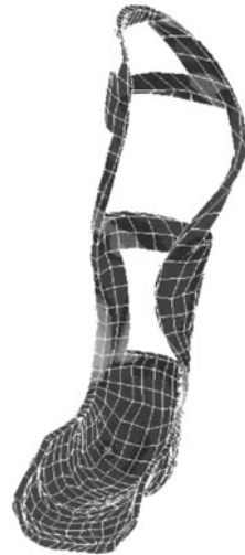
FIGURE 16.11 FEM of an ankle-foot orthotic after weight reduction. (Reprinted with permission of Khamis Abu-Hasaballah and the University of Hartford.)
