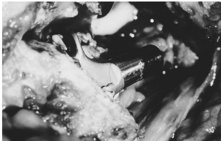
FIGURE 22.4 Fretting corrosion of the titanium Morse taper of a femoral component at revision surgery showing extensive wear. 29
