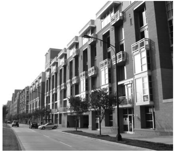
Figure 5.9 Gateway Village, Charlotte, NC, Duda Paine and David Furman, Architects, 2001. Urban design guidelines by RTKL, 1997. These mixed-use buildings in Charlotte’s city center all conform to detailed urban design guidelines that establish height, setbacks of top storeys, vertical rhythms and the requirement for pedestrian level ‘permeability’, that is, views into the ground floor uses by passing pedestrians. This communicates a sense of safety and urban activity.
