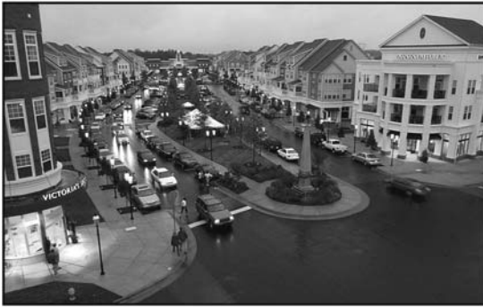
Figure 4.5 Birkdale Village, Huntersville, NC, Shook Kelly, 2002. The more relaxed spatial enclosure of this 'urban village' accommodates the car while providing generous spaces for pedestrians (see also Plates 4–7). (Photo courtesy of Crosland Inc., and Shook Kelly)
