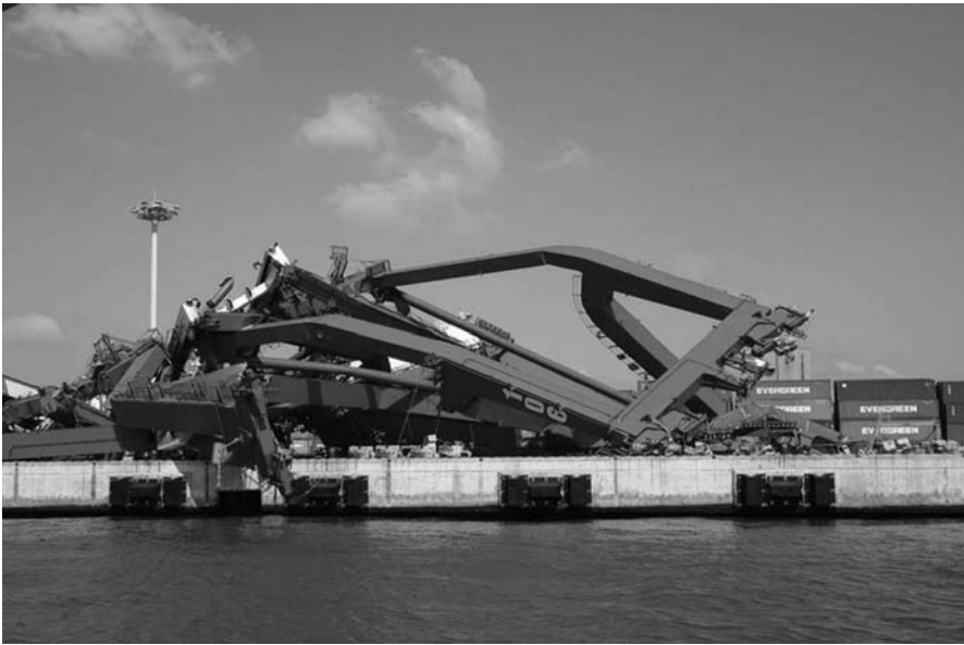
Fig. 11.1: Example of a port accident: crane collapse
