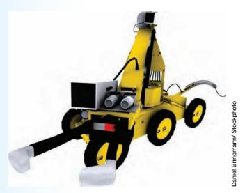
Remote-controlled robots are especially well suited for work in dangerous environments. This field robot, developed for use by bomb squads, can photograph suspicious-looking devices, move them to a safer location, and blow them up.
