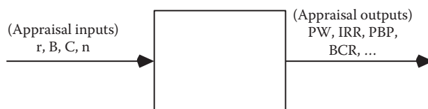
Figure 4.1 Analysis inputs and outputs. (From Carmichael, D. G., Problem Solving for Engineers , Taylor & Francis/CRC Press, London, 2013.)
