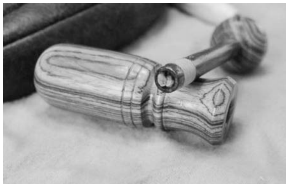
FIGURE 4.2 A modern “fire piston” based on an ancient device used by natives of the South Pacific to start fires. It is said that Rudolf Diesel was inspired to invent the diesel engine after learning of this device. (The picture is from Wilderness Solutions at http://www.wildersol.com/ . With permission of Mr. Jeff Wagner, proprietor of that company.) This picture shows the small hollow in the tip of the piston shaft where tinder is inserted prior to one quick thrust of the plunger into the wooden cylinder. This model shows the original wound string design but other models use a modern rubber O-ring. Mr. Wagner estimates temperatures of about 800°F are achieved in this wooden device.
