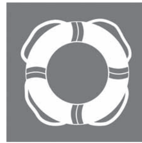
FIGURE 5.1d A green square with a white symbol signifies a safe condition sign, which is used to communicate an area of safe conditions. A green square with a white symbol is also used to signify the location of safety equipment.
