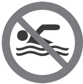
FIGURE 5.1c A red band with a red slash over a black symbol is a prohibition sign, which signifies an action not to be taken in order to avoid a hazard.
