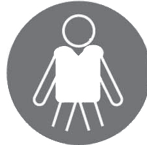
FIGURE 5.1b A blue circle with a white symbol signifies a mandatory action sign, which is used to describe an action that needs to be taken to avoid a hazard.
