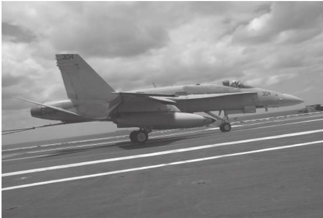
Figure 5.4 A fighter jet landing on an aircraft carrier as the tailhook captures the arresting cable. Image courtesy of Shutterstock.
