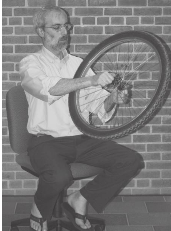
Figure 11.4 Holding a spinning bicycle wheel on a swivel chair.
