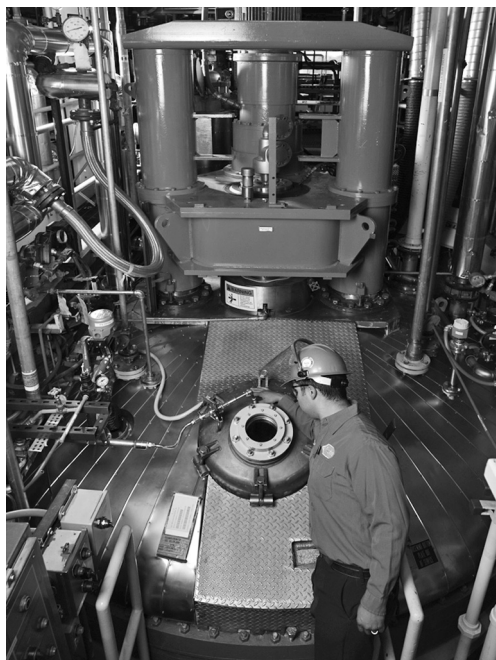
Figure 9.4 The World's largest solid phase peptide synthesizer with a volume of 10 000 L (Photo: Roche Colorado).
