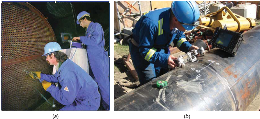
Figure 24.9 Nondestructive testing of material integrity: (a) technicians performing EDT on the tube of a nuclear plant heat exchanger. (b) A technician uses an ultrasonic phased array instrument to monitor a pipeline weld (Courtesy of David Mack/Wikimedia Commons).
