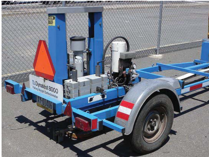
Figure 3.6 Measuring strength performance of systems—an example in highway pavements (Courtesy of Quality Engineering Solutions, Inc.).
