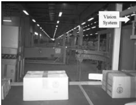
FIGURE 9-19 Vision system used in automated receiving inspection.
