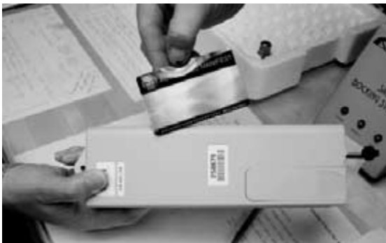
FIGURE 5-39 RF tag for container tracking and optical memory card for automated manifesting.
