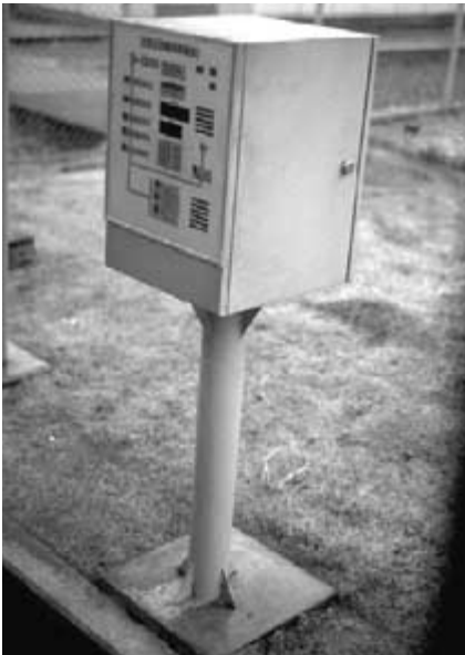
FIGURE 7-45 Voice-activated driver routing system.
