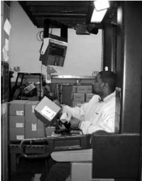
FIGURE 8-22 RF directed putaway operation.
