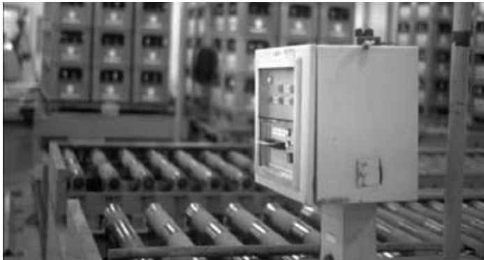
FIGURE 7-44 Smart card reader for driver-load-vehicle verification.
