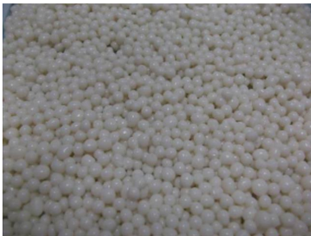
Figure 23. Photograph of fertiliserfertilizer beads obtained from natural rubber latex blended with the SA solution.
