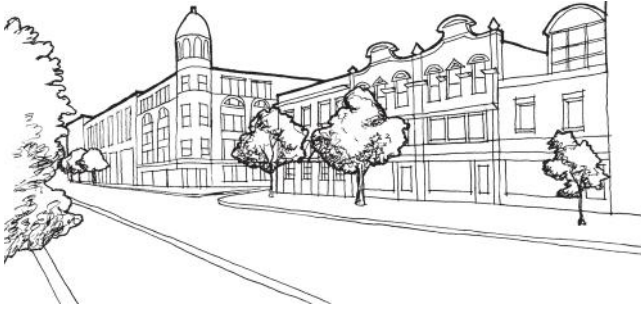
FIGURE 2.14 This sketch utilizes line weight to communicate the distance edges and contours are from one another. The outer contours of objects are therefore the thickest lines in the drawing.
