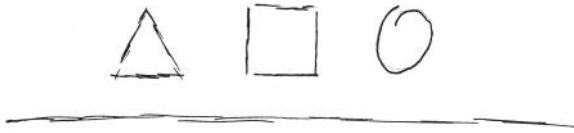
FIGURE 2.10 These are examples of how not to draw lines or shapes in architectural sketches. Chicken scratch lines and hurried shapes can distract from the meaning of a drawing.
