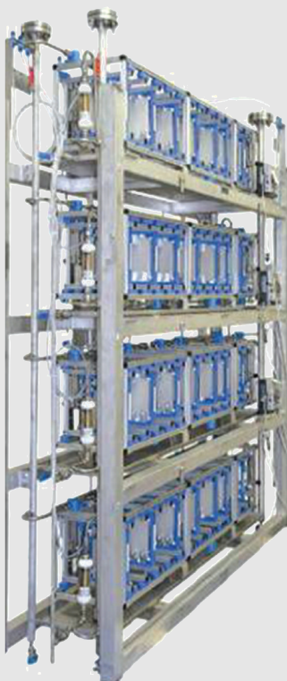
Figure B14.6.2 Production bank, containing four identical reactor lines in parallel. Two such production banks enable a production capacity of up to 1000 t/a. Courtesy of Corning.
