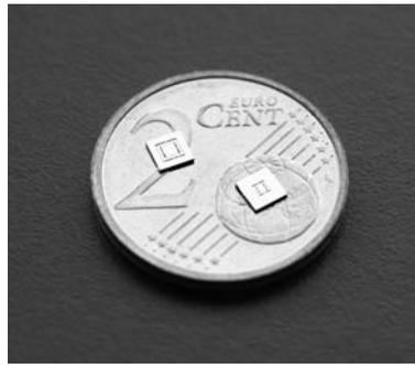
**Figure 6.9** Silicon-based two-dimensional scanning micromirrors on a 2-cent coin, with two differing mirror sizes. The chip sizes for both are  $3 \times 3$  mm. Photo courtesy of Khaled Aljaseem.
