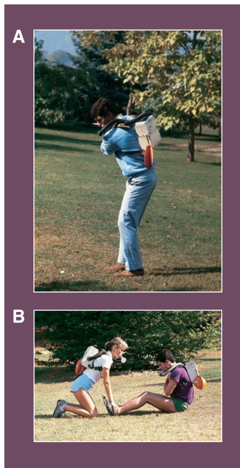
FIGURE 6.4 ■ Portable spirometer to measure oxygen uptake by the open-circuit method during (A) golf and (B) calisthenics exercise.
