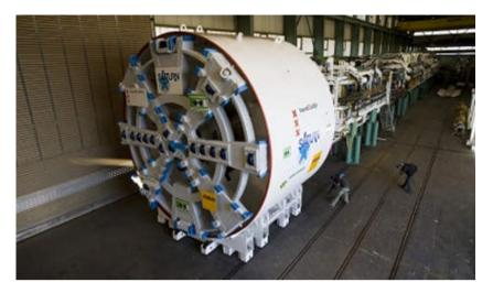
Figure 4.1. Drilling head of equipment used by Bouygues for the Amsterdam metro. (Source: AD, December 8, 2009.)
