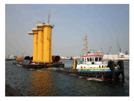
Figure 19.2. Sea transport of three wind turbine foundations with sub-piles for wind farm under construction. Best risk allocation is on a knock-for-knock basis. (Photo: SMIT, www.smit.com/tugmagazine/june2011.)
