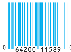
FIGURE 2-3 An example of the universal product code (UPC), which is often preprinted on the labels of retail products for merchandise identification and computerized checkout.
