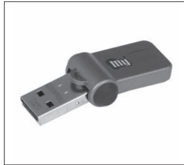
FIGURE 2-13 This USB flash drive from AData corporation plugs into a standard USB connector on a microcomputer. Despite its small size, it stores 1 gigabyte of data. Source: ADATA Technology (USA) Co., Ltd.
