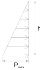
FIGURE 3.4 Water pressure diagram.
