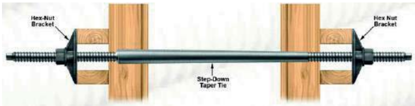
FIGURE 9.14 Taper tie cross section.
