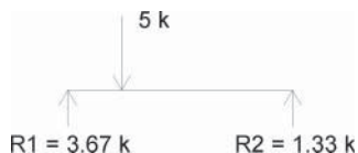
FIGURE 1.21 Simple beam resultant force solution.
