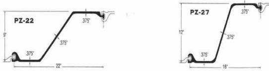
FIGURE 7.2A Hot rolled sheet pile.
