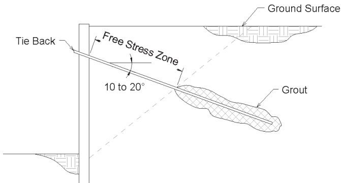
FIGURE 6.22 Soil anchor embedded behind failure plane.
