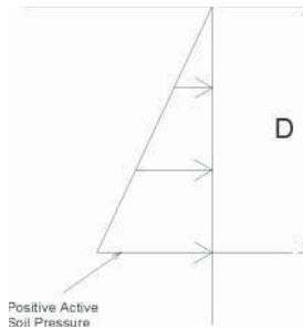
FIGURE 5.8 Active soil pressure diagram.
