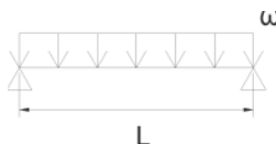
FIGURE 6.3 Typical loading diagram for lagging.
