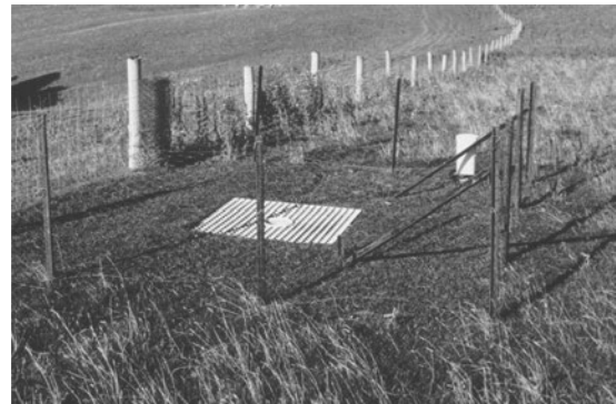
Figure 2.7 Surface rain gauge with non-splash surround.
