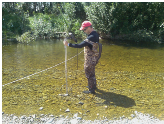
Figure 8.5 Portable ADCP (SonTek Flow Tracker) being used to measure a small stream.
