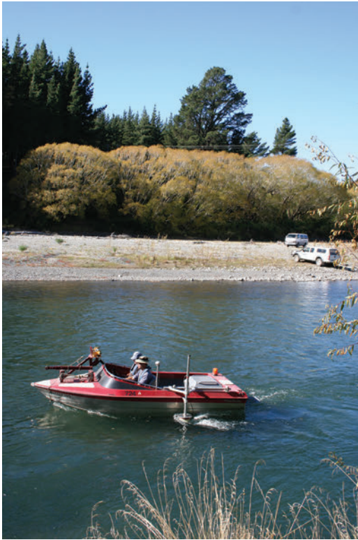
Figure 8.6 A boat mounted ADCP carrying out a cross section. The disc at the bottom of the pole on the near side of the boat (just touching the water surface) is the ADCP sensor.
