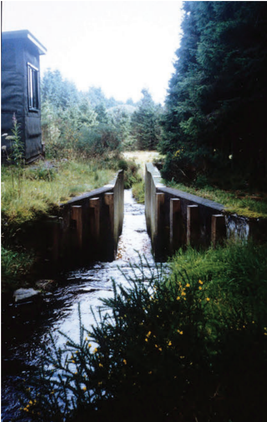
Figure 8.19 A trapezoidal flume. The stream passes through the flume and the water level at the base of the flume is recorded continuously.
