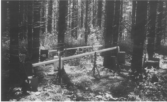
Figure 4.6 Throughfall troughs sitting beneath a pine tree canopy. This collects rain falling through the canopy over the area of the trough. It is sloping so that water flows to a collection point.
