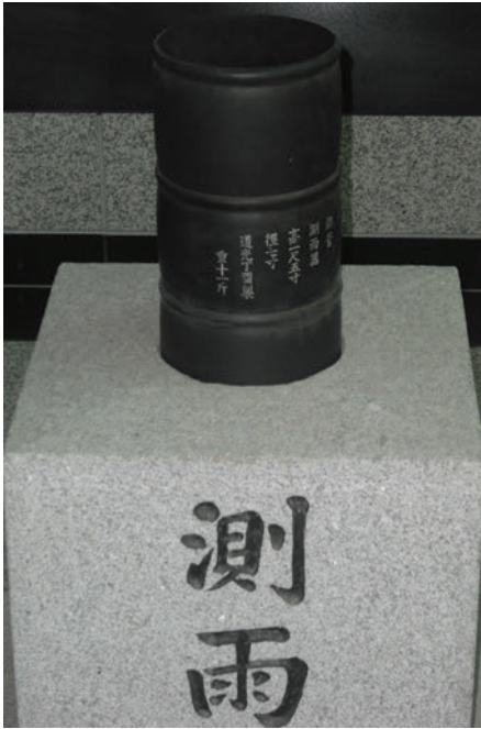
Figure 2.6 (a) A fourteenth-century rain gauge from Korea. Photo: Tim Davie. (b) A rain gauge sitting above the surface to avoid splash.
