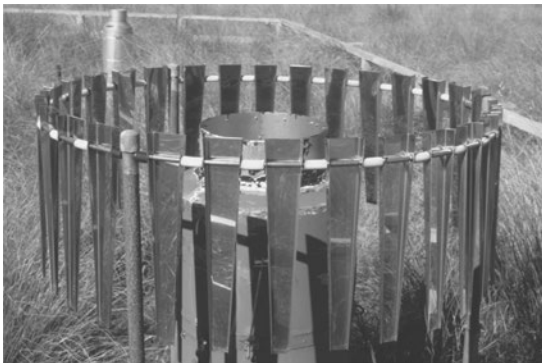
Figure 2.9 Baffles surrounding a rain gauge to lessen the impact of wind turbulence. The gauge is above ground because of snow cover during the winter.
