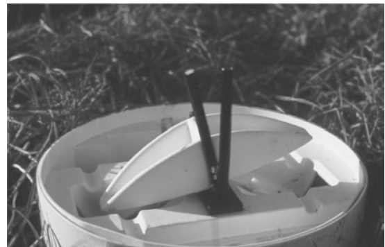
Figure 2.11 The inside of a tipping-bucket rain gauge. The 'buckets' are the small white, triangular reservoirs. These are balanced and when full they tip over, bringing the black arm past the other stationary arm. In doing so a small electrical current is passed to a data logger.
