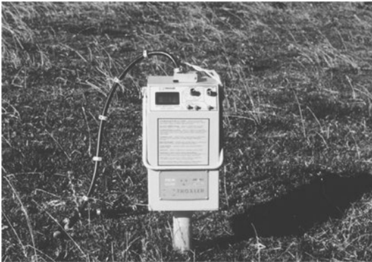
Figure 6.15 A neutron probe sitting on an access tube. The black cable extends down into the tube with the source of fast neutrons (and counter) at the tip.
