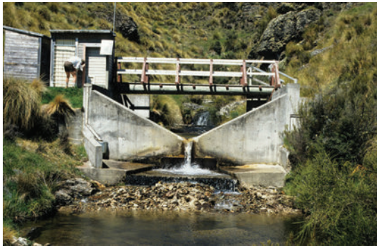
Figure 8.18 A V-notch weir. The water level in the pond behind the weir is recorded continuously.
