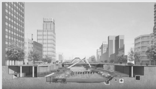
Figure 11.15 Schematic diagram of Cheonggyecheon restoration project, showing infrastructure as well as the river.
