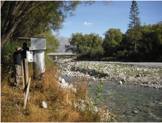
Figure 8.10 A hydrometric station with the stilling well beside a gravel bed river.
