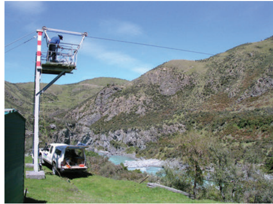
Figure 8.4 Cableway used for gauging in a large river. The current meter is suspended from the cable at set points across the river and a velocity profile is measured.
