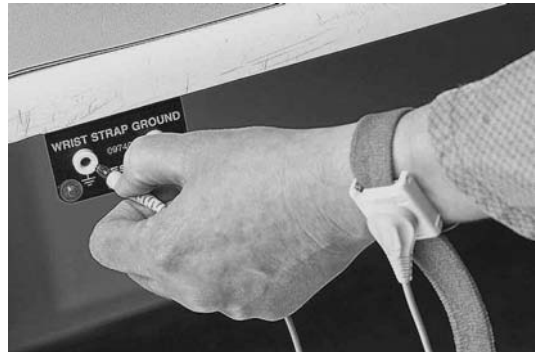
12.6 Using a wrist strap for a bench operation (note the grounding jack connector)
